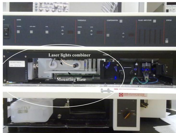
Figure 69: Laser lights combiner mounted on an adjustable base. Three laser lights can align collinearly.
