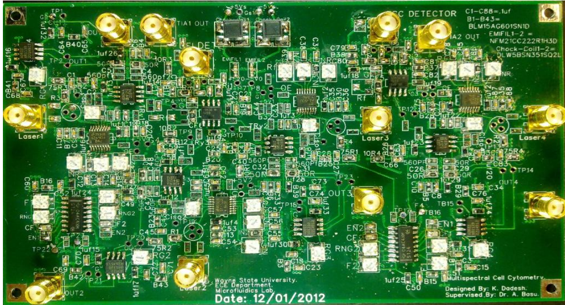
Figure 50: PCB layout for the FDM system. All components are surface mount technology (SMT). Four laser drivers, model EL6245 (Elantec), with up to 500 MHz sinusoidal oscillators onboard are used to modulate laser diode currents. They can be driven using four external square wave voltage controlled oscillators, SN74S124D. Two low noise amplifiers with 1.6 GHz gain-bandwidth product are used to amplify the detected multiplexed high frequency light signals. Four 500 MHz analogue multiplier, AD834 (Analog Devices), and four low pass filters are used as heterodyne demodulators for each channel. Four instrumentation amplifiers, AD622 (Analog-Devices), are used to amplify the four DC differential outputs. Input and output signals can be accessed via SMA connectors. Variable SMT resistors are used to adjust modulation frequencies and amplitudes.
