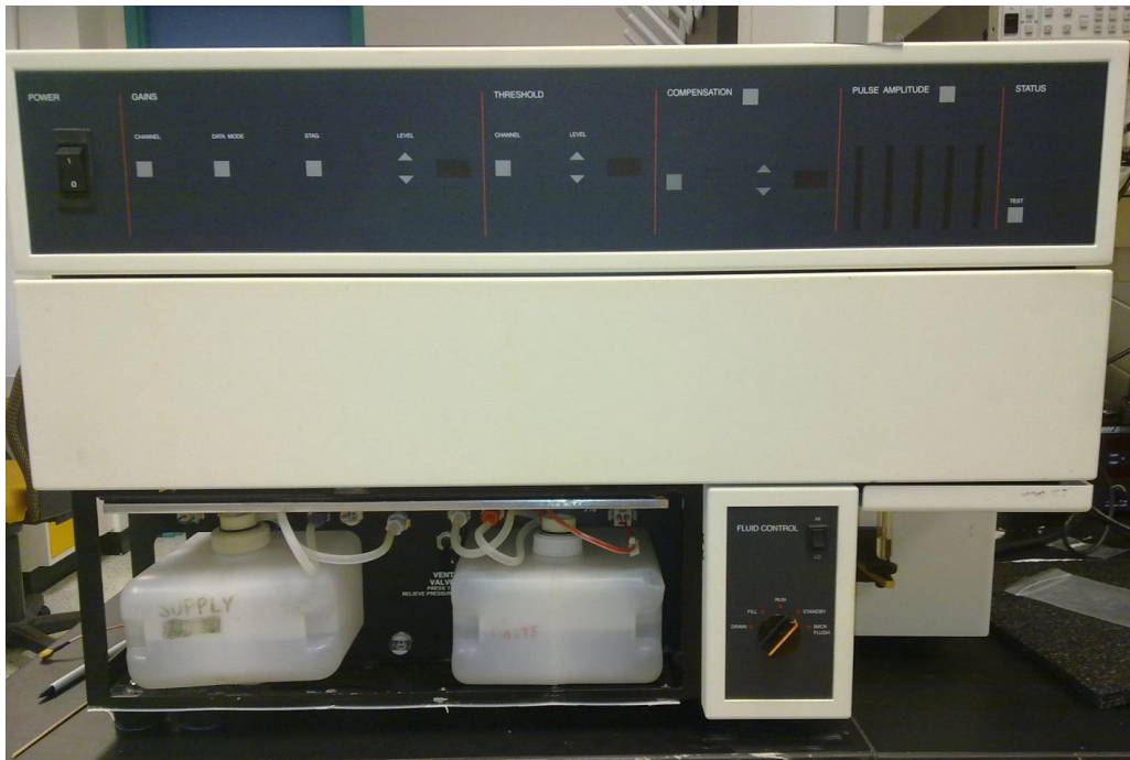
Figure 61: An old BD Immunocytometry system model FACScan. It has had a malfunctioning laser light source, and all other parts are completely functioning.
