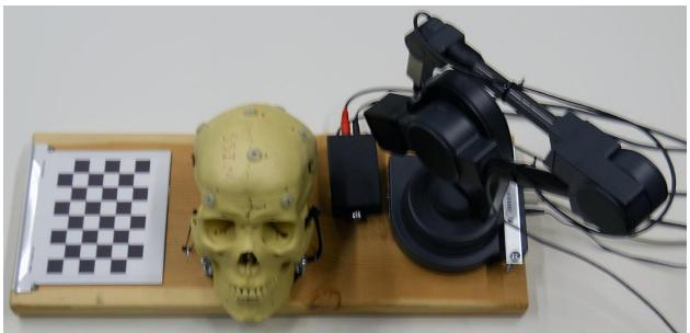
Figure 36: Hardware testbed for AR system
