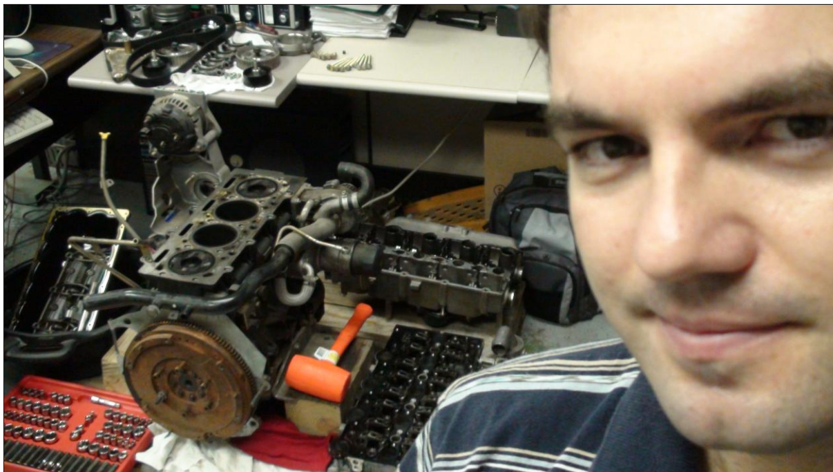
Figure 3.14b - VM Motori 2.5 L engine dismantled in order to draw its moving parts
