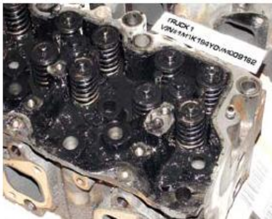
Figure 1.5 - B20 valve deck sludge accumulation according to Richard Fraer et.al. [6]
