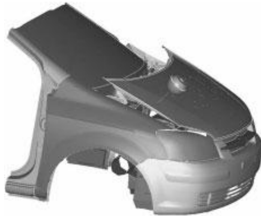
Figure 5.2.1: concept of active hood system (Huang and Yang, 2009)
