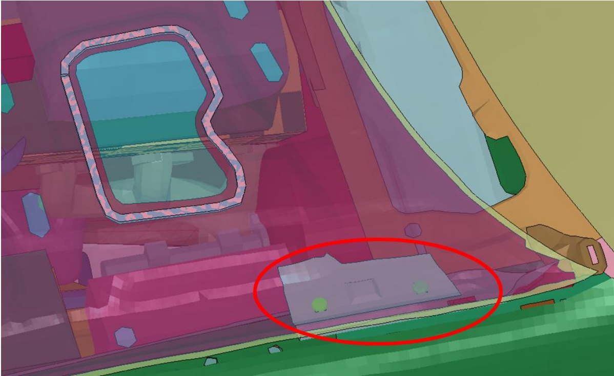
Figure A.7: Rear Hinges modeled in details with actual bolts
