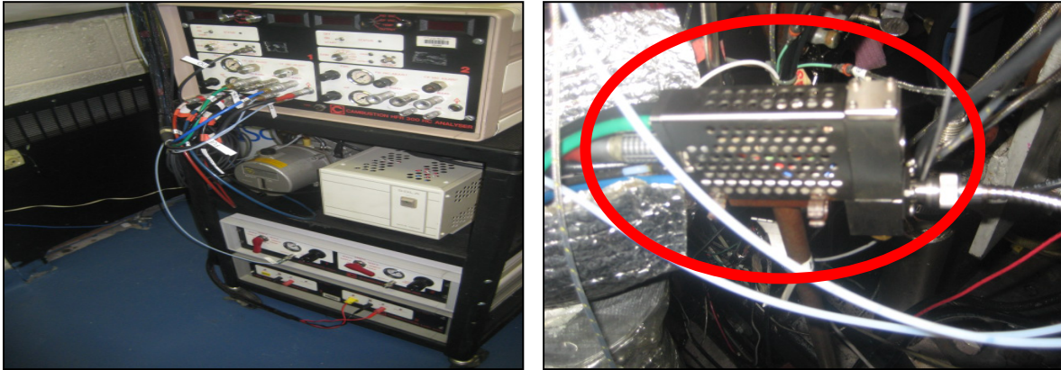
Figure 2.23 – Fast response FID.
