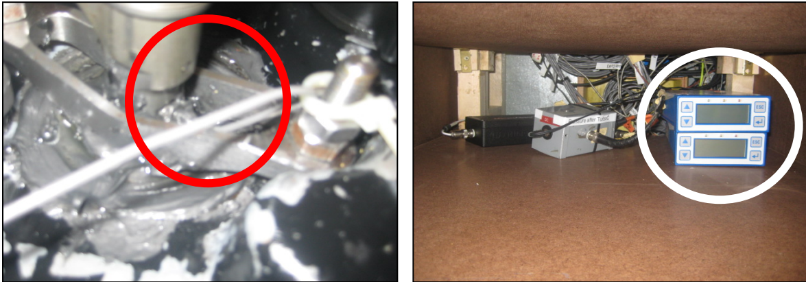
Figure 2.16 – Needle lift sensor and its charge amplifier.
