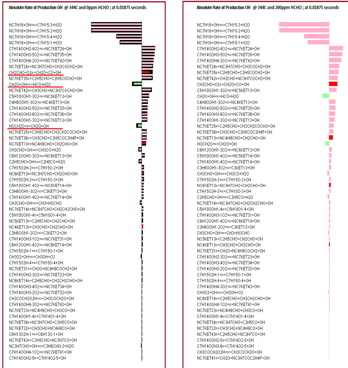
Figure 4.33.b - Comparison using superposition between the rate of formation of OH at 0.018750 seconds with zero and 200ppm HCHO
