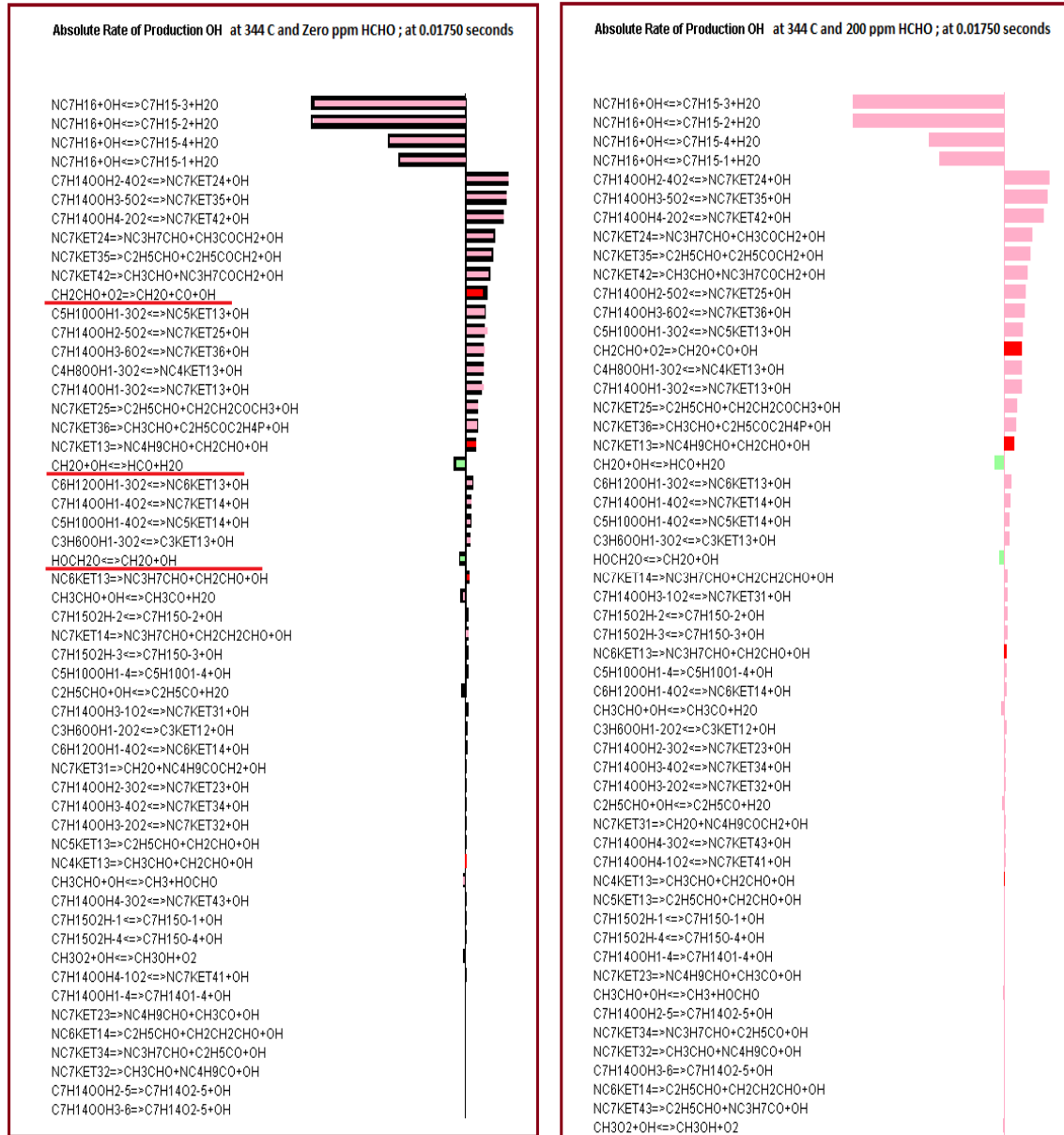
Figure 4.30.b - Comparison using superposition between the rate of formation of OH at 0.01750 seconds with zero and 200ppm HCHO
