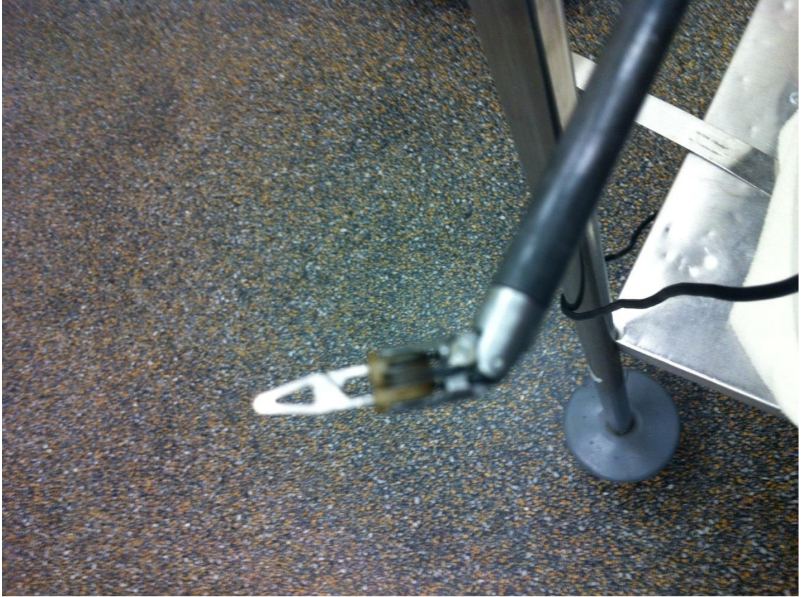
Figure 17. One of the micro-instruments inserted through the trocars, showing multiple joints and swivels on the “hand.”
