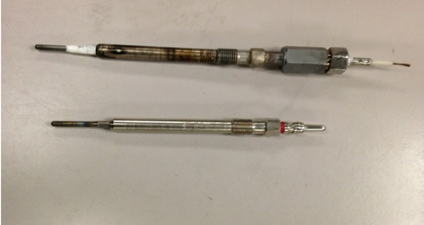
Figure 3-19. Original glow plug and integrated glow plug/ion sensor prototype used for research.
