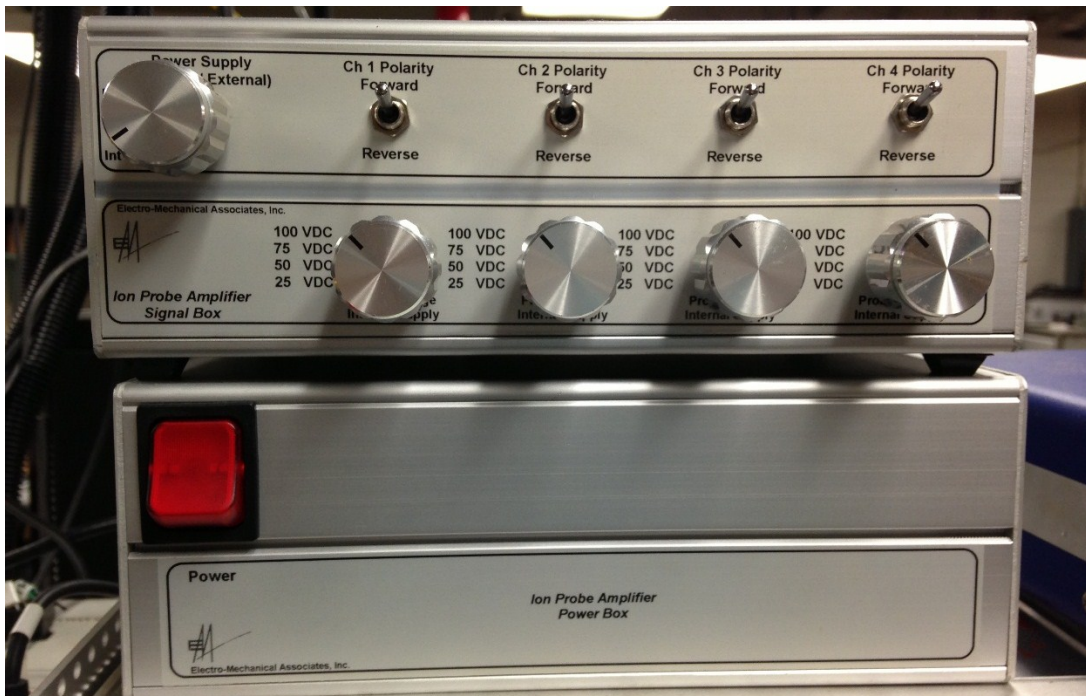
Figure 3-17. Ion current measuring circuit
