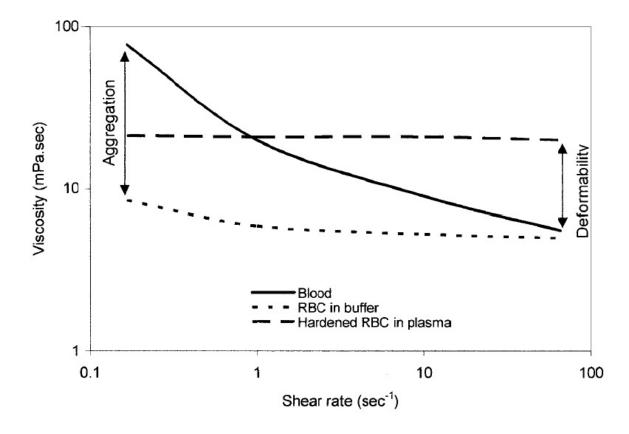
Figure 5: Relationship between the viscosity of blood and the shear rate [6]
