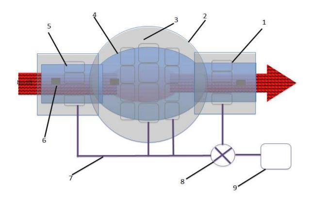
Figure 13: A pneumatic version of the pumping apprentice. (1) outgoing sphincter valve controlled by pneumatic cuff, outer titanium case, (3) main pump pneumatic cuff actuator, (4) polymer pump body with PEO lining, (5) inlet sphincter valve cuff, (6) 6-axis accelerometer chips for actuation analysis, (7) pneumatic control lines, (8) valve to control actuation, (9) pneumatic pump (saline or gas).
