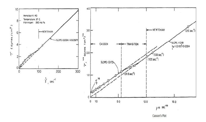
Figure 4: Non- Newtonian shear stress and shear strain rate along with Casson's Plot [8]
