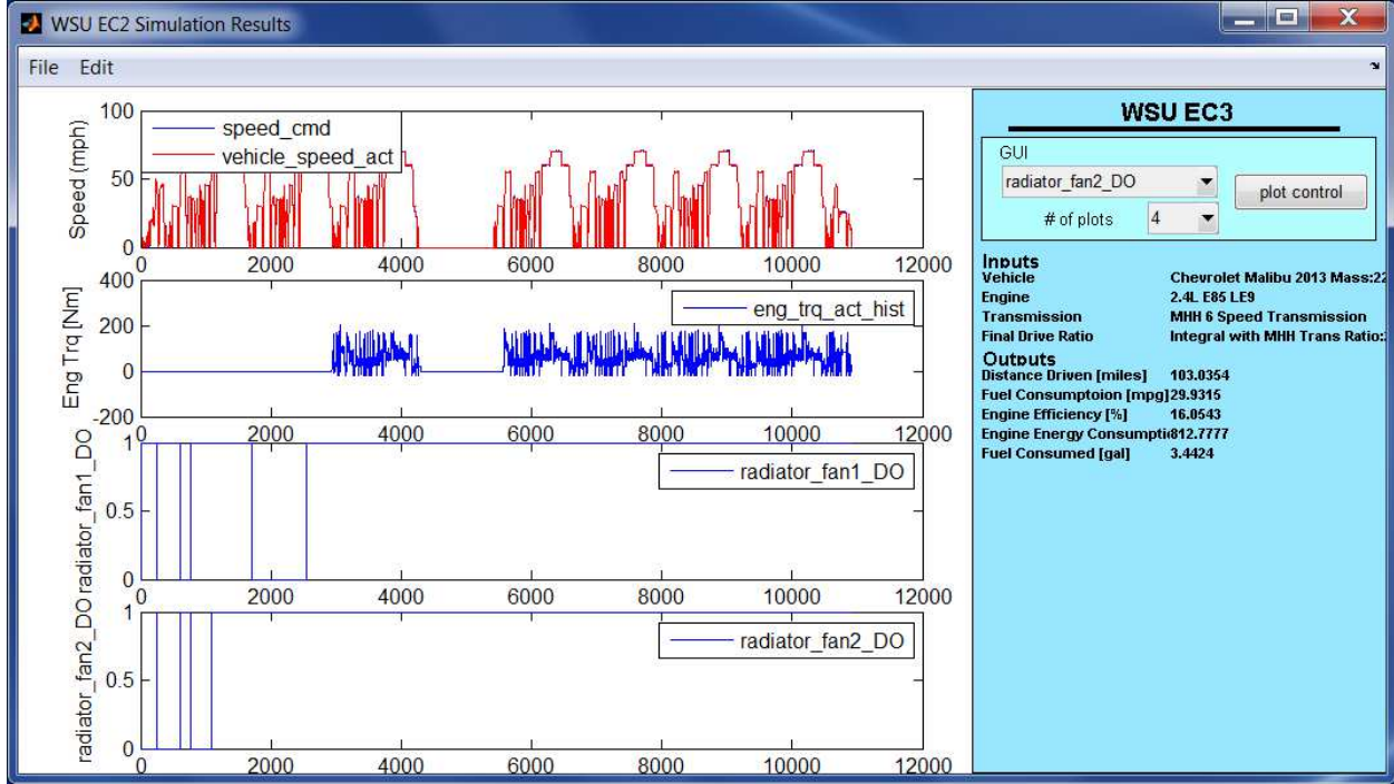
Figure 3-68. Motor thermal model advancement: radiator fan speed command data is now visible in simulation results.
