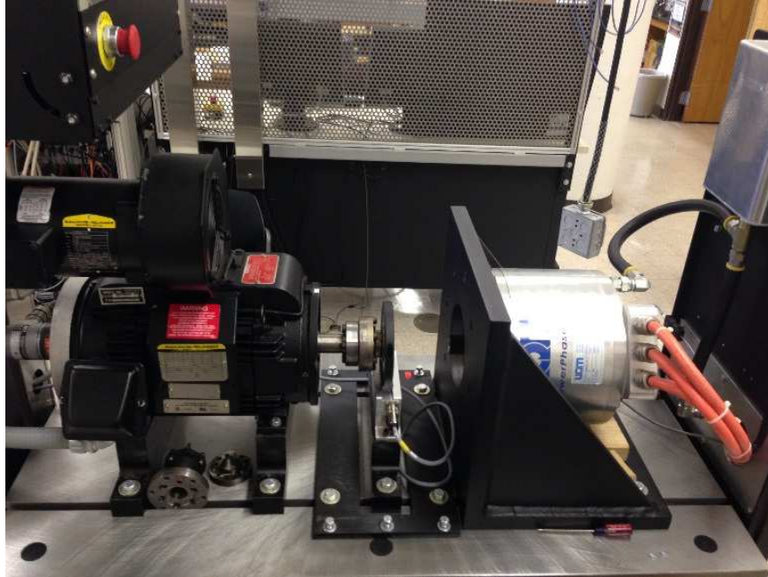
Figure 3-4. Motor dyno stand with 20 kW induction AC motor (painted black, on left) for dyno load. The UQM Technologies motor (on right) was the original Device Under Test (DUT).
