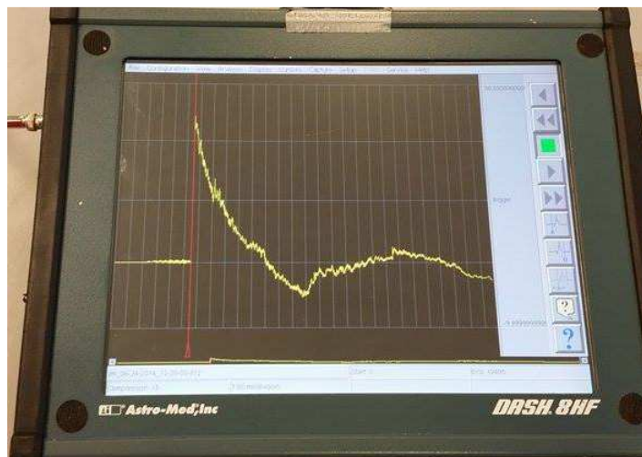
Figure 22: Image showing the driver pressure of 22psi on the DASH system.
