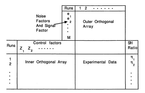
Figure 4.2. Inner & outer orthogonal arrays for dynamic characteristic.
