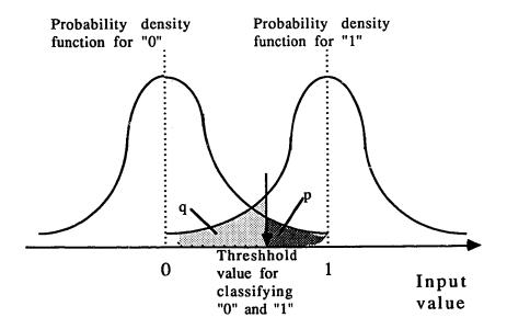
Figure 5.2. Distribution of the input variable for  $p\neq q$
