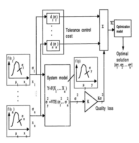
Figure 6.2. Optimization for tolerance design
