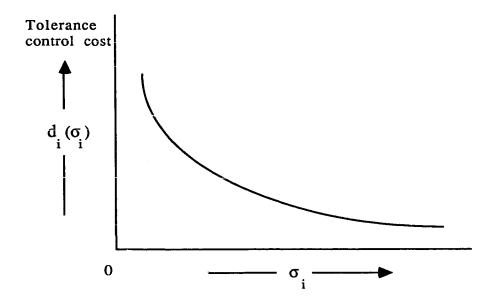
Figure 6.1. Tolerance control cost vs tolerance  $\sigma_i$
