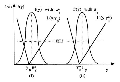
Figure 2.5. E[L] remains unchanged when moving f(y) and  $L(y,y_0)$  simultaneously
