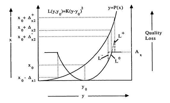
Figure 7.6. The tolerances for the lower-level characteristic x.
