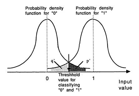
Figure 5.3. Distribution of the input variable for p'=q'
