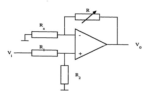
Figure 4.4. A noninverting amplifier.
