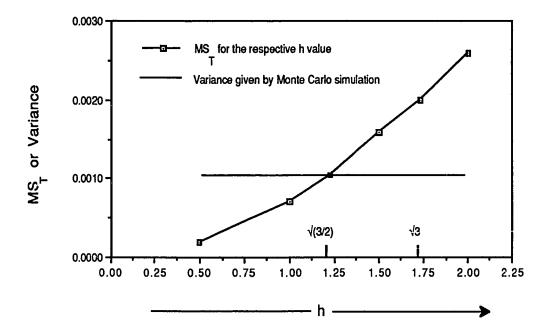
Figure 6.3. The comparison of  $\sigma_y^2$  and  $MS_T$  for various h values (The result of the Monte Carlo simulation is based on 2000 times of simulation and the assumption that all noise factors are normally distributed).
