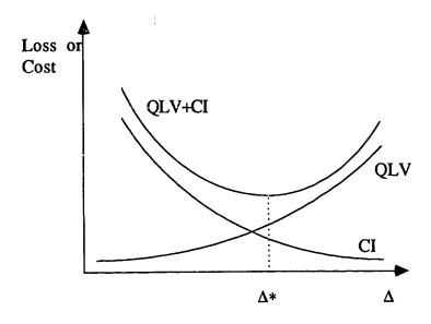
Figure 7.1. Balance of quality loss due to variations and cost increase due to control of tolerances.
