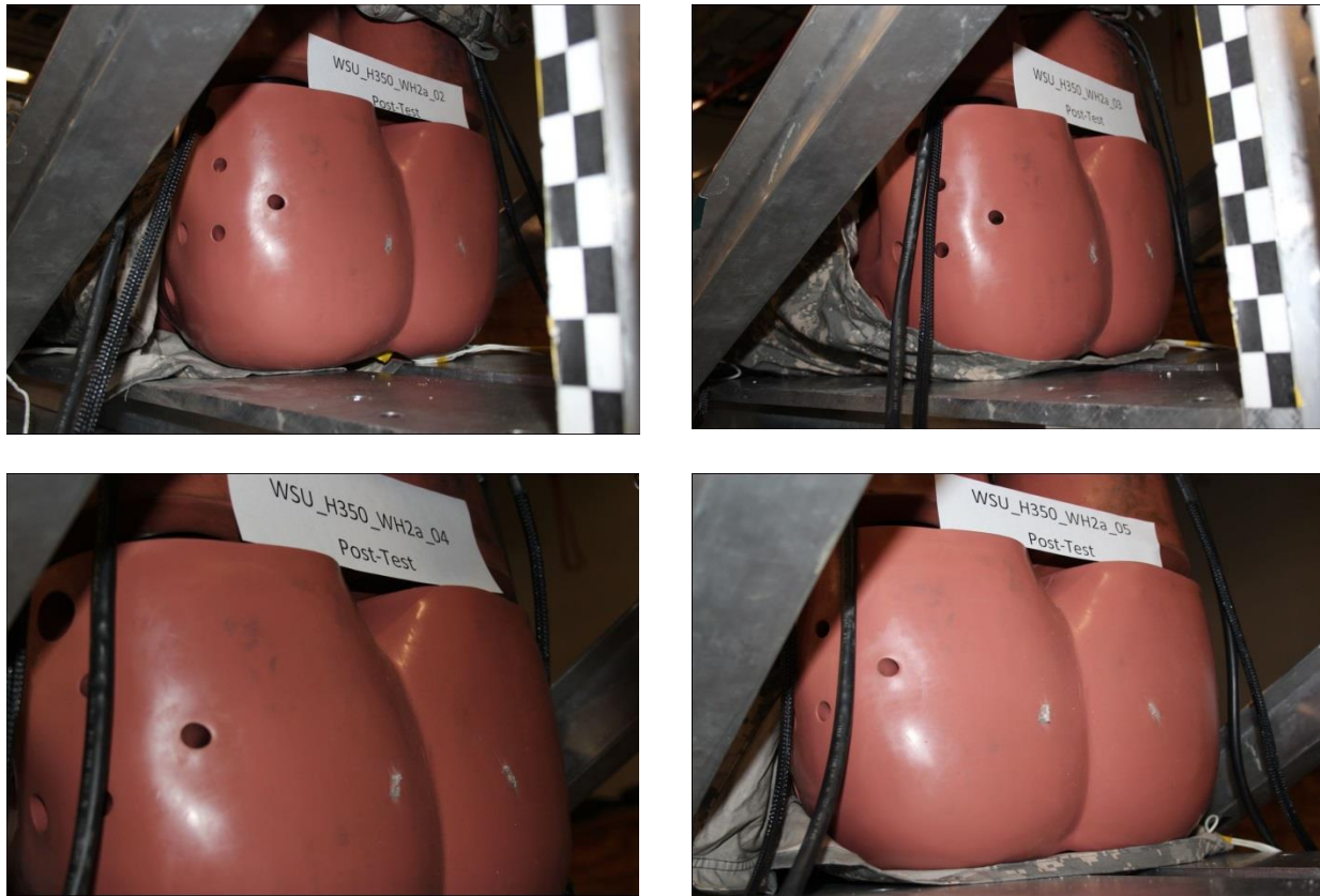
Figure 6-11: Snapshot showing the punctured pelvis flesh impacted with loading condition 2. After the first experiment the rupture worsen with additional tests.
