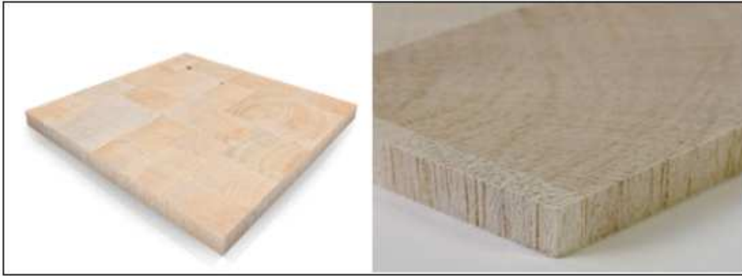
Fig. 4.2. End-grain balsa wood
