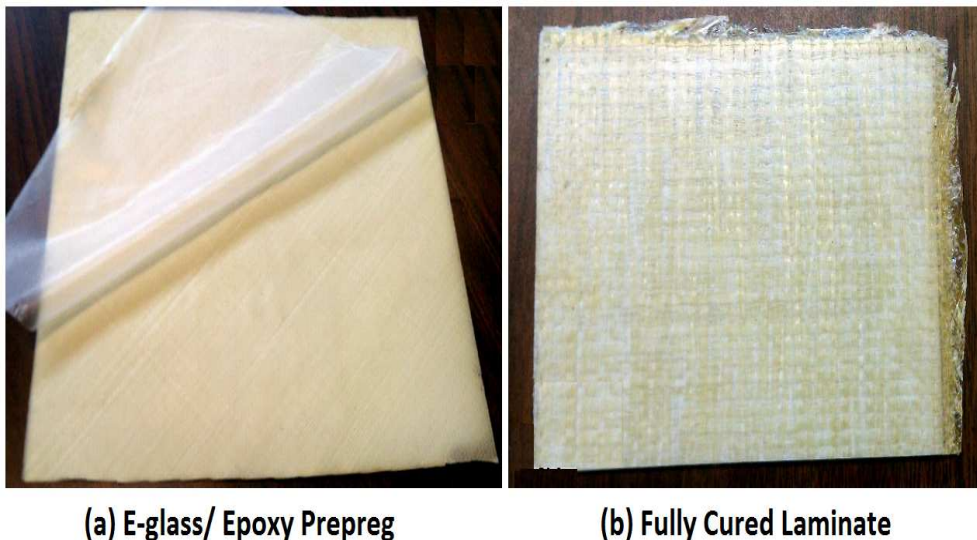
Fig. 4.1. Prepreg material and fully cured laminate
