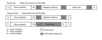
Figure 2.6: I2C Interface Concept diagram [37]
