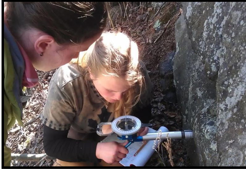
Figure 2. Student Lauren Schraeder orienting a drilled sample using the Pomeroy Orienting Fixture with a Brunton Compass installed.
