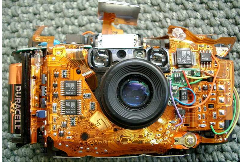
Figure 1.1. Flexible PCB inside an Olympus Stylus camera. From: Steve Jurvetson http://flickr.com/photos/44124348109@N01/2265519 .
