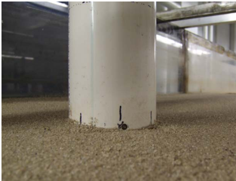
Figure 3.17: Initial bed condition and initial pressure port exposure
