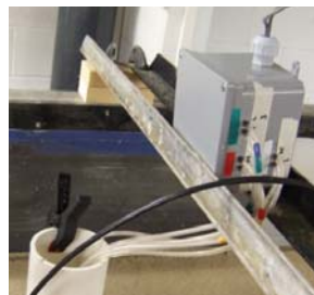
Figure 3.15 b) Pressure sensor assembly
