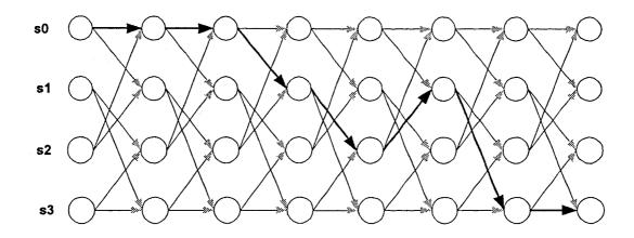
Fig(4b) Trellis diagram showing a sample of data stream
