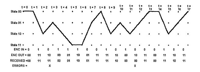
Fig(9) Encoded message with a couple of bit errors
