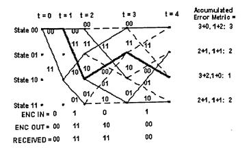
Fig(13) The trellis diagram between t = 0 and t = 4
