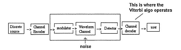
Fig(1) A model of digital communication system
