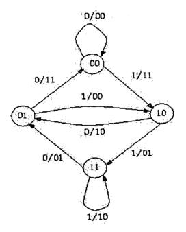
Fig(3) The state transition diagram for the K = 3, r = 1/2 convolutional encoder
