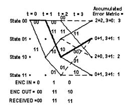
Fig(12) The trellis diagram between t = 0 and t = 3
