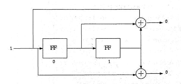
Fig(2) An example of a 1/2 rate convolutional encoder with K=3 (4 states)
