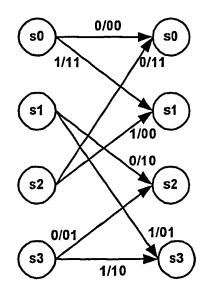
Fig(4a) A window of the trellis diagram showing a sample of data stream
