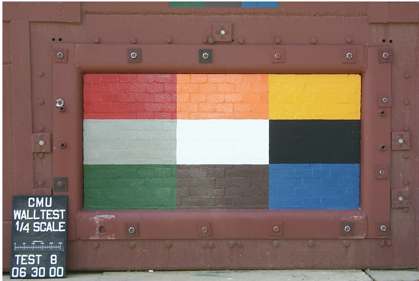
Figure 2. Experimental Set-up. Pressure gauges are the four small white circles on frame outer perimeter; one on top and two on each side (fifth hidden by test placard in lower left corner).
