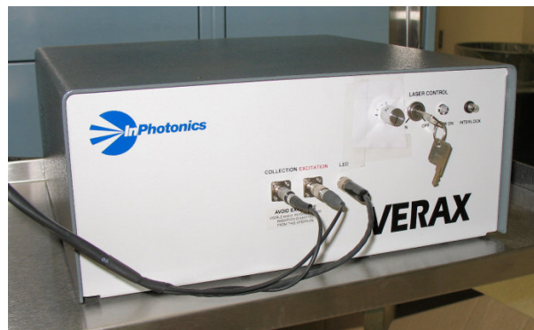
Figure 4.3: The VERAX portable Raman spectrometer with an attached fiber optic probe.
