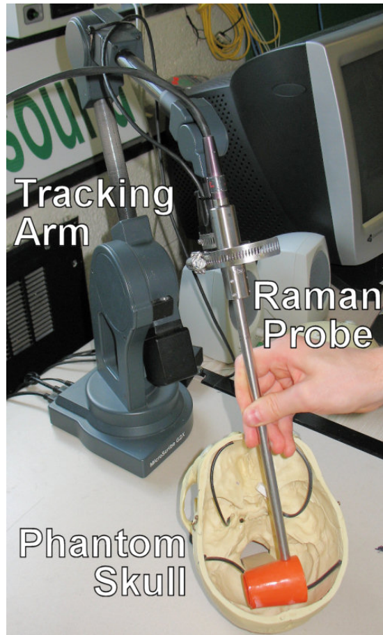
Figure 4.2: The Raman probe, attached to the end of the tracking arm, is used to scan a plastic cup and other objects within the phantom skull.
