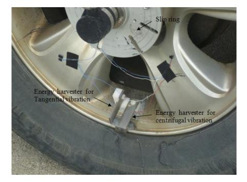
Figure 5.12. The road test assembly on the wheel for centrifugal and tangential vibration simultaneously.
