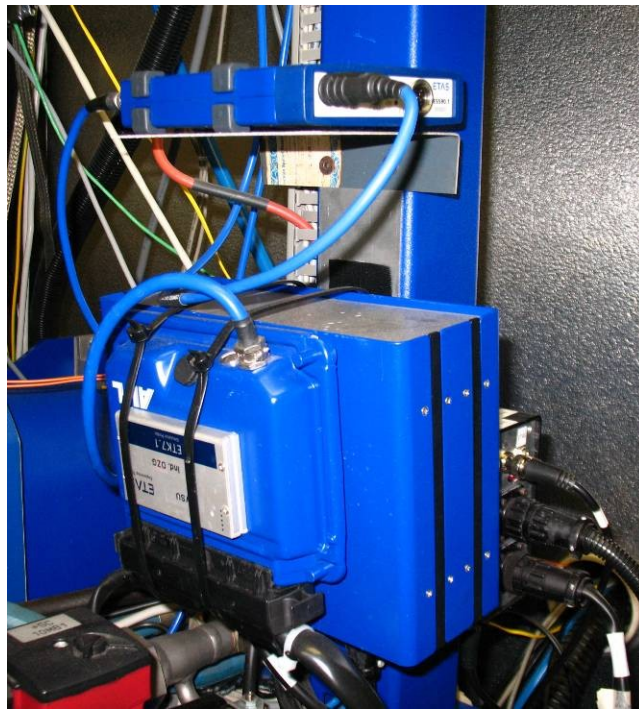
Fig 4.7 – Bosch ECU and ETAS VTK7.1
