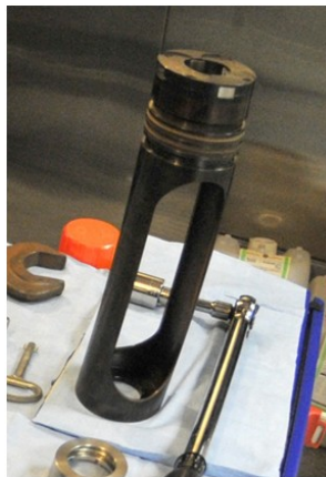
Fig 4.2 – Elongated optical piston
