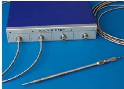
Fig 2.10 – AVL sensor installed in glow plug adapter [89]
