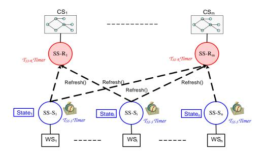
Figure 5.6: Fault Coordinators.
