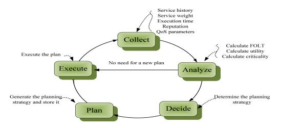
Figure 3.2: The autonomic control loop for FLEX.
