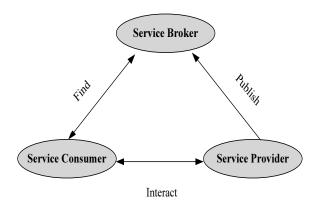
Figure 1.1: Service-Oriented Interaction Model.
