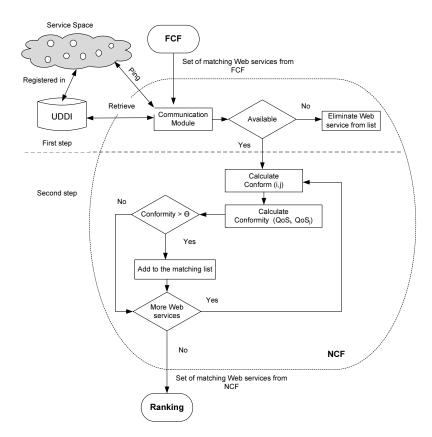
Figure 4.8: Non-functional Filter (expanded).
