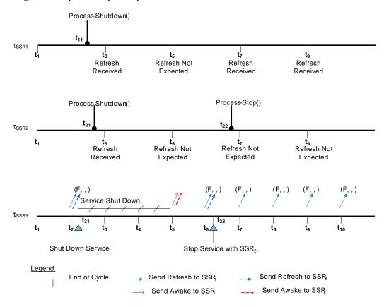
Figure 5.14: Removal-SS Protocol - Example.
