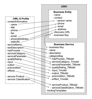
Figure 4.4: Mapping between OWL-S and UDDI constructs.
