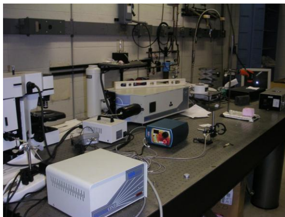
Figure B.14 The Raman spectroscopy was used in this study, including Jobin–Yvon Horiba Triax 550 spectrometer, a liquid-nitrogen cooled charge-coupled device (CCD) detector, an Olympus model BX41 microscope with a 100 \times objective, and a Modu-Laser (Stellar-Pro-L) Argon-ion laser operating at 514.5 nm.
