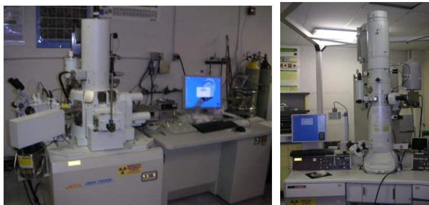
Figure B.2 The SEM (JOEL 7600F)-left and TEM (JOEL 2010)-right were used for characterizing the nano structure and chemical elements of materials.
