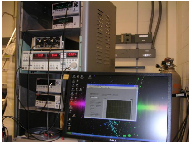
Figure B.13 The AC measurement setup includes lock-in amplifier, current pre-amplifier, volt and current meters together with Labview software to control the system.
