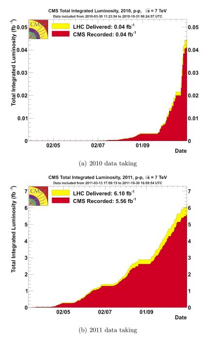
FIG. 3.5. Integrated luminosity delivered to (yellow), and recorded by CMS (red) for 2010 and 2011 p–p runs at  $\sqrt{s}=7$  TeV.
