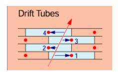
FIG. 3.16. Muon drift tube operation. The red line with arrow shows a muon traversing the drift tube. The anode wires (shown by red dots) are perpendicular to the page. The horizontal blue lines with arrows show the muon's distance from the anode wire (obtained by multiplying the speed of an electron in the tube by the drift time).
