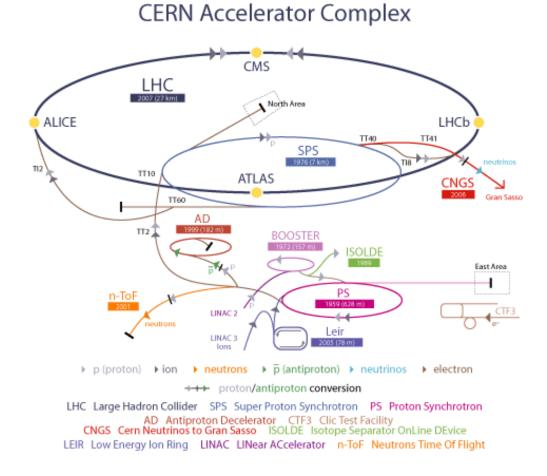
FIG. 3.2. Layout of the CERN accelerator complex [60].
