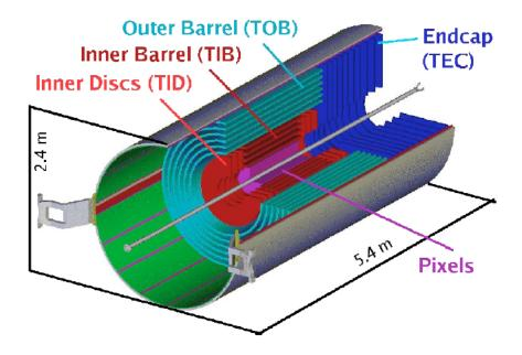
FIG. 3.9. Layout of the CMS inner tracking system [55].
