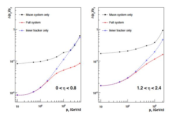
FIG. 3.21. The muon  $p_T$  resolution as a function of  $p_T$  using simulated data for the muon system only, the inner tracking system only, and both [55]. Left panel:  $|\eta| < 0.8$ , right panel:  $1.2 < |\eta| < 2.4$ .
