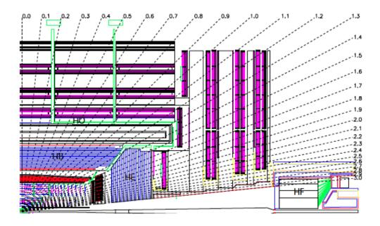
FIG. 3.13. Layout of the hadron calorimeter [55].
