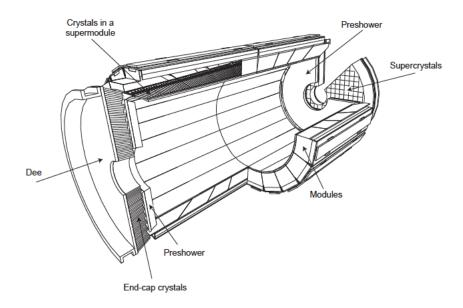
FIG. 3.12. Layout of the CMS ECAL showing the arrangement of PbWO<sub>4</sub> crystals in the barrel and endcap regions, along with the preshower detector [55]
