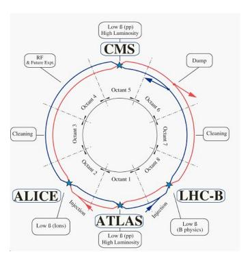
FIG. 3.1. Schematic layout of the LHC collider tunnel [53].
