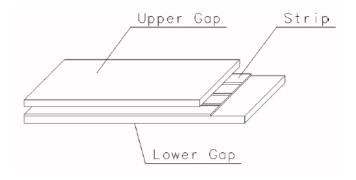
FIG. 3.20. Layout of a double-gap RPC [55].
