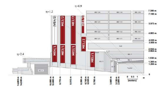
FIG. 3.17. Quarter-view of the CMS detector [55]. Shown in red color are the CSCs. The  $\rm ME4/2$  chambers will eventually be built and installed as part of the CMS upgrade plans.
