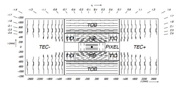
FIG. 3.10. Schematic layout of the CMS tracker showing detailed coverage in the r-z plane [55]. Each line represents a detector module. Double lines indicate back-to-back modules which deliver stereo hits.
