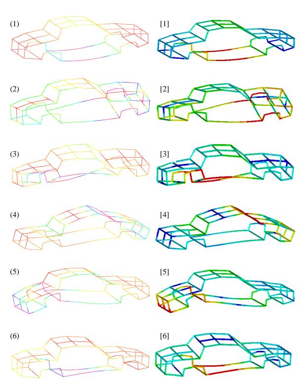
Figure 5.13 The first six mode shapes of the car frame from current method ( left side and indexed in parenthesis) and FEM method with 2173 elements (right side and indexed in square bracets)
