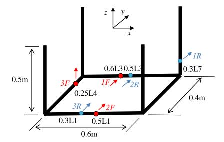
Figure 5.5 A scheme showing the input force and response locations.
