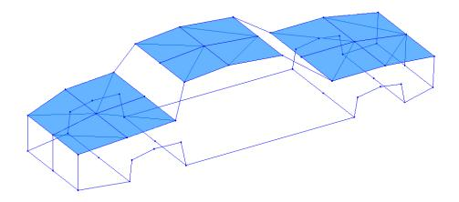
5.8.4 Example 4: a car frame structure with coupled roof side plates
