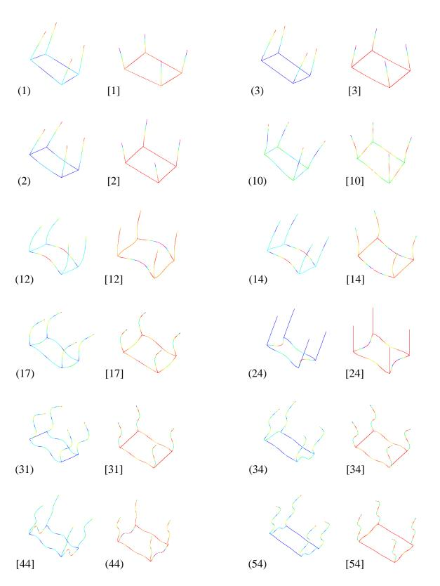
Figure 5.9 Some typical low to mid frequency mode shapes from current method (mode numbers in parentheses) and FEM method (mode numbers in brackets).
