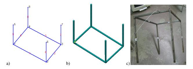
Figure 5.4 A rigidly connected 3-D frame. a) Setup used in current method with corner numbers at the frame corners and beam numbers in the middle of the beams. b) FEM model c) Lab setup with the same number sequence as current and FEM models.
