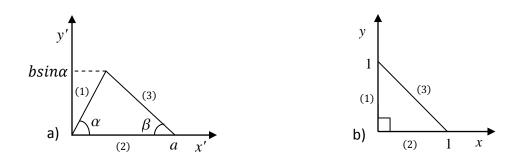
Figure 5.3 A triangular plate before (a) and after (b) coordinator transformation
