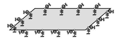
Figure 3.1 A rectangular plate elastically restrained along all the edges
