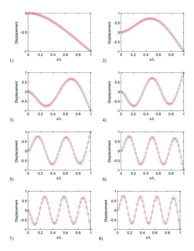
Figure 2.2 The first eight lowest mode shapes for a cantilever beam obtained by current method with truncation number M=10 (blue curves) and by the exact solution equation (red circles).
