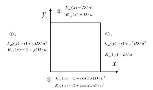
Figure 3.4. A rectangular plate with varying elastic edge supports including linear, parabolic, and harmonic functions.
