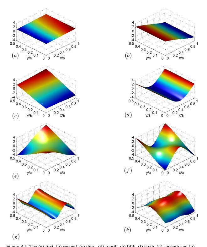
Figure 3.5. The (a) first, (b) second, (c) third, (d) fourth, (e) fifth, (f) sixth, (g) seventh and (h) eighth mode shapes for a plate with aspect ratio r = 2 and boundary condition described in Figure 3.4.
