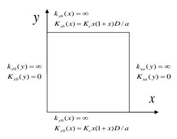
Figure 3.3 A simply supported plate with rotational springs of parabolically varying stiffness along two opposite edges, where  $K_c$  is a constant.
