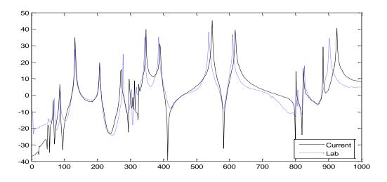
Figure 5.8 FRF curves of the 3-D frame with input force at 0.25L of beam 4 in z direction and response measured at 0.3L of beam 1 in y direction.
