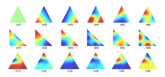
Figure 4.3. The first six mode shapes of a free equilateral triangular plate as described in Section 4.6.1 (a1-a6), a right-angled isosceles triangular plate with elastic boundary constraints k = 10 and K = 100 as described in Section 4.6.3 (b1-b6), and an anisotropic plate with  $\beta = 30^{\circ}$  and elastic boundary constraints k = 100 and K = 50 as described in Section 4.6.4 (c1-c6).
