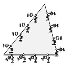
Figure 4.1. A general triangular plate with elastically restrained edges.
