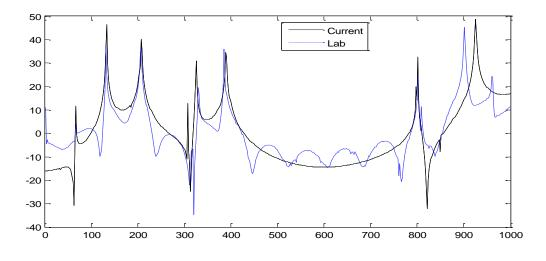
Figure 5.7 FRF curves of the 3-D frame with input force at 0.5L of beam 1 in y direction and response measured at 0.3L of beam 5 in y direction.
