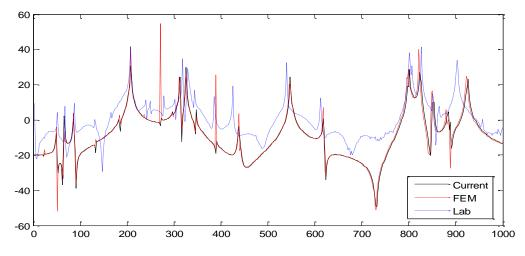
Figure 5.6 FRF curves of the 3-D frame with input force at 0.6L of beam 3 in y direction and response measured at 0.3L of beam 7 in y direction.
