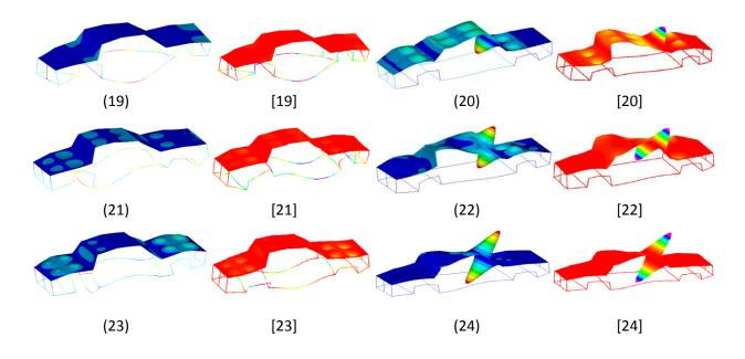
Figure 5.15 The first twenty four mode shapes of the car structure obtained by using FEM method (left side and indexed in parenthesis ) and current FSEM method (right side and indexed in square brackets)
