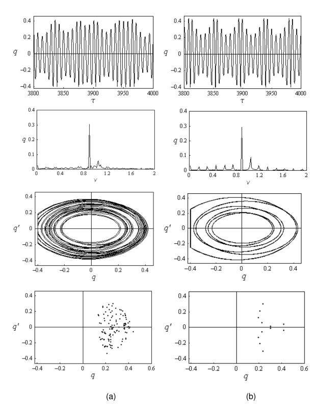
Figure 4.3. Time History Records, FFT, Phase portraits, and Poincaré Maps for v = 0.88, and a = 0.06. Initial conditions  $z_o = 0.11$ ,  $z_o' = -0.19$ . (a) Elastic impact e = 1, and (b) Inelastic impact (Model 1) e = 0.8.
