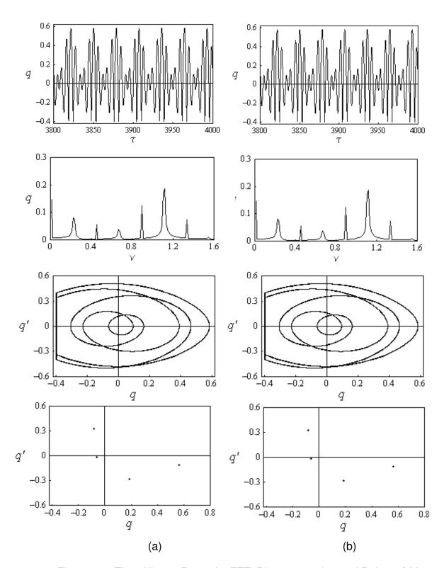
Figure 4.5. Time History Records, FFT, Phase portraits, and Poincaré Maps for v = 0.88, and a = 0.084. Initial conditions  $z_o = 0.01$ ,  $z_o' = 0.03$ . (a) Elastic impact e = 1, and (b) Inelastic impact (Model 1) e = 0.8.
