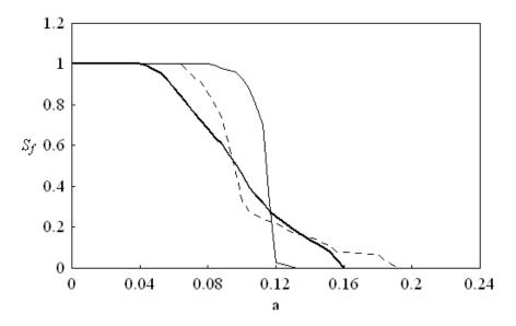
Figure 3.23. Dependence of stability fraction on excitation amplitude for three different values of excitation frequency -v = 0.88, -v = 0.94, -v = 1.2.
