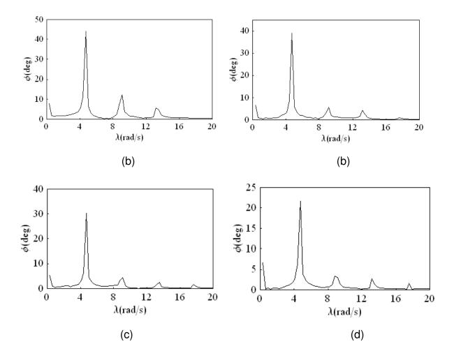
Figure 5.23. FFT plots of the model response of Figure 5.22. under motor speed  $N_m = 2.2 \text{ rad/s}$ : (a) in the absence of barrier, (b) in the presence of one-sided barrier at  $-40^\circ$ , (c) at  $-30^\circ$ , and (d) at  $-20^\circ$ .
