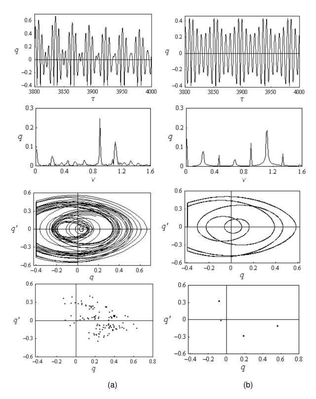
Figure 4.4. Time History Records, FFT, Phase portraits, and Poincaré Maps for v = 0.88, and a = 0.084. Initial conditions  $z_o = 0.15$ ,  $z_o' = 0.31$ . (a) Elastic impact e = 1, and (b) Inelastic impact (Model 1) e = 0.8.
