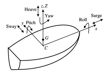
Figure 2.1. Ship Schematic diagram showing the six degrees of freedom.
