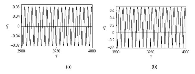
Figure 3.17 Section of time history response records for excitation frequency ratio v = 1.2, and excitation amplitude: (a) a = 0.036, and (b) a = 0.088.
