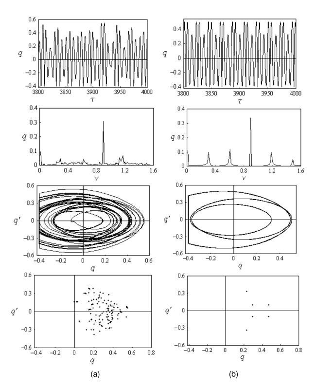
Figure 4.8. Time History Records, FFT, Phase portraits, and Poincaré Maps for v = 0.88, and a = 0.104. Initial conditions  $z_o = 0.15$ ,  $z_o' = 0.09$ . (a) Elastic impact e = 1, and (b) Inelastic impact (Model 1) e = 0.8.
