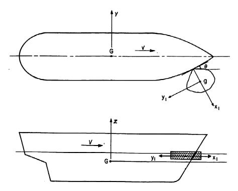
Figure 1.4. Ice floe-ship impact by Aboulazm (1989).
