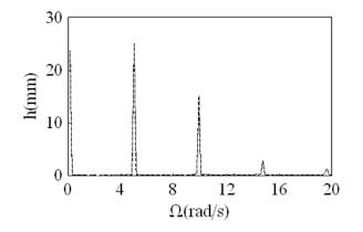
Figure 5.30. FFT of excitation waves corresponding to Experimental record, and ----- Fourier series representation.
