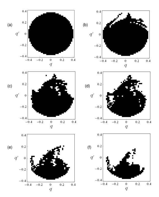
Figure 4.15. Domains of attraction for different excitation amplitudes for v = 1.2 as predicted by Model 1 for inelastic impact (e = 0.8); (a) a = 0.04, (b) a = 0.064, (c) a = 0.096, (d) a = 0.104, (e) a = 0.12, and (f) a = 0.136; Black region: bounded (safe) motion, and empty space: rollover dynamics.
