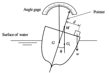
Figure 5.2. Inclination experiment to determine the metacentric height.
