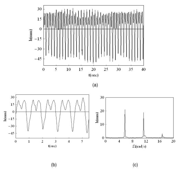
Figure 5.16. Free surface wave at wave maker motor speed  $N_m = 2.8$  rad/s : (a) time history record of the water free surface, (b) magnification of few cycles showing the wave profile, and (c) FFT plot.
