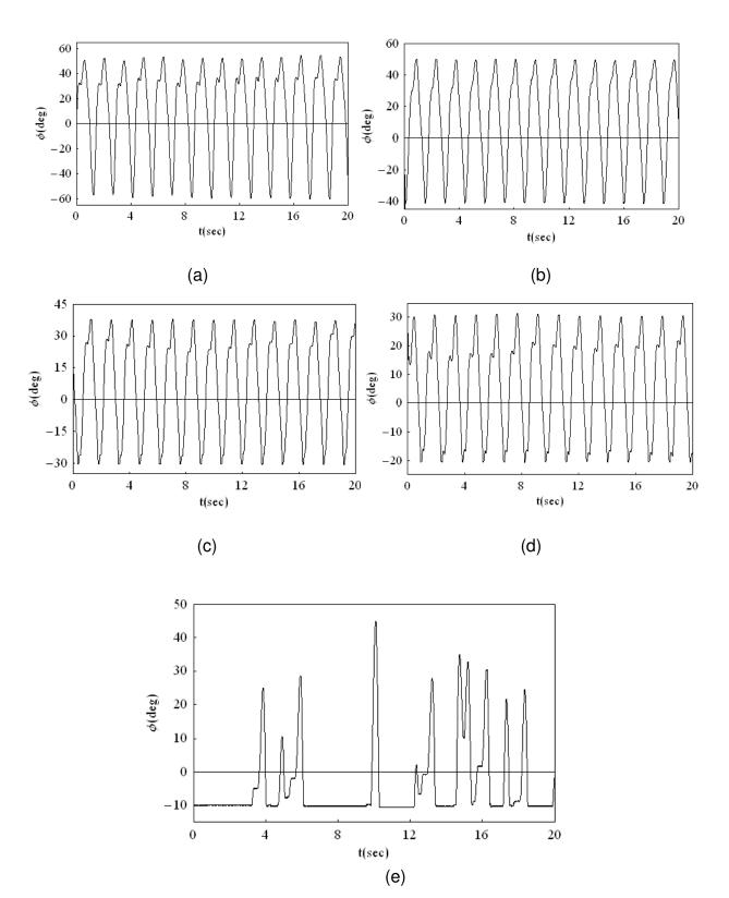
Figure 5.22. Measured time history records of the model response under motor speed  $N_m = 2.2 \text{ rad/s}$ : (a) in the absence of barrier, (b) in the presence of onesided barrier at  $-40^\circ$ , (c) at  $-30^\circ$ , (d) at  $-20^\circ$ , (e) at  $-10^\circ$ .
