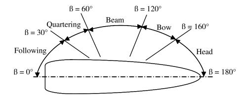
Figure A.2. Definition of incident wave directions.
