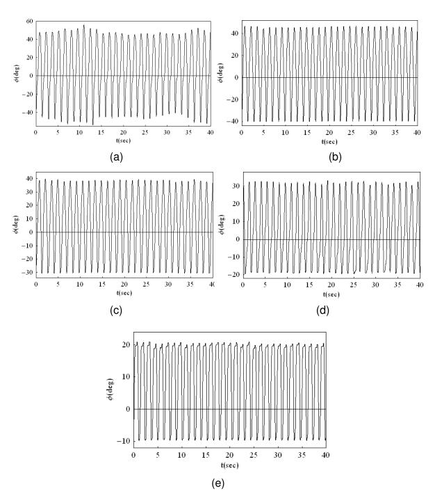
Figure 5.13. Measured time history records of the model response under motor speed  $N_m = 2.4$  rad/s : (a) in the absence of barrier, (b) in the presence of onesided barrier at  $-40^\circ$ , (c) at  $-30^\circ$ , (d) at  $-20^\circ$ , (e) at  $-10^\circ$ .
