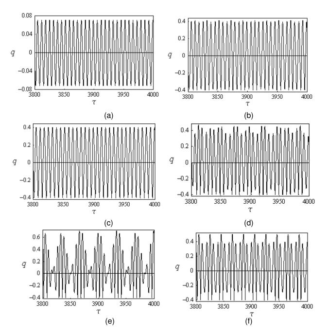
Figure 3.11 Section of time history response records for excitation frequency ratio v = 0.94, and excitation amplitude: (a) a = 0.008, (b) a = 0.04 (period-two), (c) a = 0.06, (d) a = 0.07, (e) a = 0.096, and (f) a = 0.12 (period-three).
