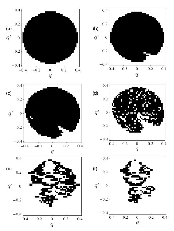
Figure 3.9. Domains of attraction for different excitation amplitudes for excitation frequency v = 0.88 : (a) a = 0.04, (b) a = 0.096, (c) a = 0.10, (d) a = 0.112,
