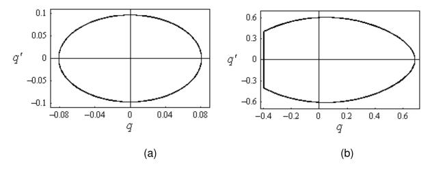
Figure 3.19. Phase portraits corresponding to the time history records of Figure 3.17 for excitation frequency ratio v = 1.2, and excitation amplitude: (a) a = 0.036, and (b) a = 0.088.
