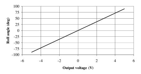
Figure 5.9. Calibration curve of the magnetic angle sensor.
