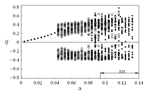
Figure 3.10. Bifurcation diagram for excitation frequency ratio v = 0.88. Period-one response,  $\Diamond$  Modulated response,  $\Box$  Multi - periodic response, • Chaotic motion, and RM= Rollover Motion.
