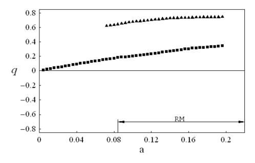
Figure 4.29. Bifurcation diagram for v = 1.2 as predicted by Model 2 for inelastic impact (e = 0.8); Period-one response, A Period-one response experiencing impact, and RM= Rollover Motion.
