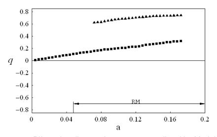
Figure 4.16. Bifurcation diagram for v = 1.2 as predicted by Model 1 for inelastic impact (e = 0.8); Period-one response, A Period-one response experiencing impact, and RM= Rollover Motion.
