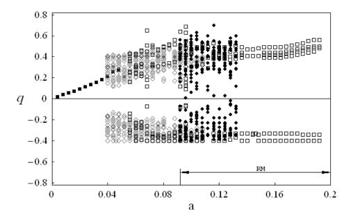
Figure 4.12. Bifurcation diagram for v = 0.88 as predicted by Model 1 for inelastic impact (e = 0.8); Period-one response,  $\diamond$  Modulated response,  $\Box$  Multi - periodic response,  $\bullet$  Chaotic motion, and RM= Rollover Motion.
