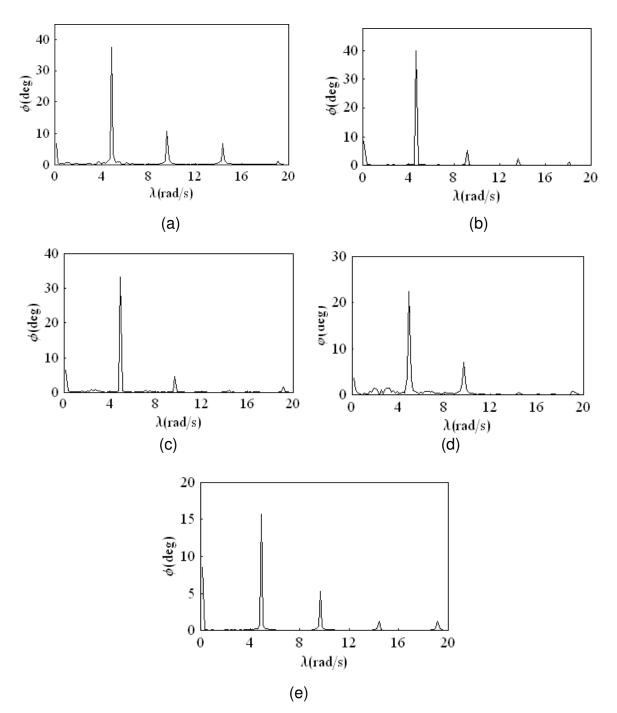
Figure 5.14. FFT plots of the model response of Figure 5.13. under motor speed  $N_m = 2.4 \text{ rad/s}$ : (a) in the absence of barrier, (b) in the presence of one-sided barrier at  $-40^\circ$ , (c) at  $-30^\circ$ , (d) at  $-20^\circ$ , (e) at  $-10^\circ$ .
