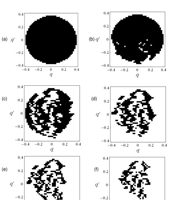
Figure 4.11. Domains of attraction for different excitation amplitudes for v = 0.88 as predicted by Model 1 for inelastic impact (e = 0.8); (a) a = 0.08, (b) a = 0.104, (c) a = 0.12, (d) a = 0.14, (e) a = 0.16, and (f) a = 0.18; Black region: bounded (safe) motion, and empty space: rollover dynamics.
