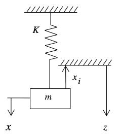
Figure 1.6. Spring-mass system with one sided barrier.
