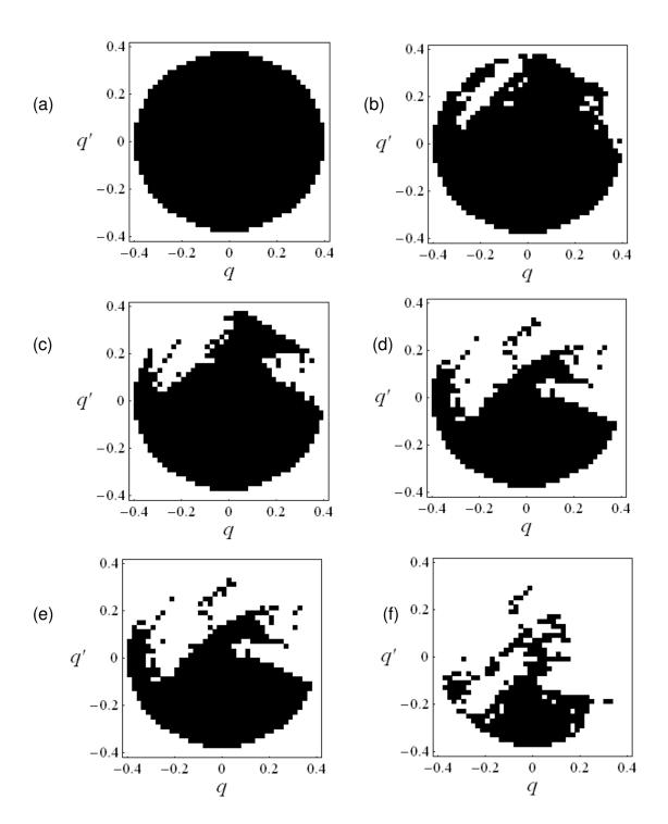
Figure 4.28. Domains of attraction for different excitation amplitudes for v = 1.2 as predicted by Model 2 for inelastic impact (e = 0.8); (a) a = 0.04, (b) a = 0.096, (c) a = 0.104, (d) a = 0.12, (e) a = 0.136, and (f) a = 0.144; Black region: bounded (safe) motion, and empty space: rollover dynamics.
