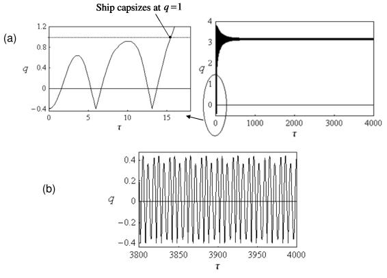
Figure 4.9. Time History Records for v = 0.88, and a = 0.104. Initial conditions  $z_o = 0.65$ ,  $z_o' = -0.23$ ; (a) Elastic impact e = 1, and (b) Inelastic impact (Model 1) e = 0.8.
