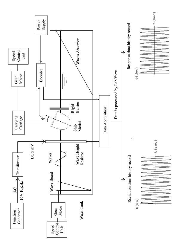
Figure 5.5. Block diagram showing the experiment layout.
