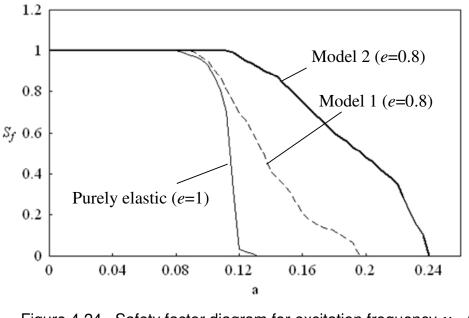
Figure 4.24. Safety factor diagram for excitation frequency v = 0.88; \_\_\_\_\_Purely elastic impact (*e*=1), and inelastic impact(*e*=0.8); \_\_\_\_\_Model 1, and \_\_\_\_\_Model 2
