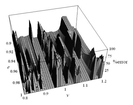
Figure 4.47. Error involved in equivalent damping method as a function of excitation frequency ratio v and coefficient of restitution e for a = 0.08,
