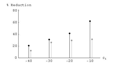
Figure 5.26. % Reduction in response amplitude vs impact angle. Black:  $N_m = 2.4$  rad/s , and Gray:  $N_m = 2.8$  rad/s .
