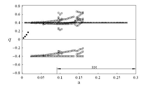
Figure 4.26. Bifurcation diagram for v = 0.94 as predicted by Model 2 for inelastic impact (e = 0.8); Period-one response, A Period-one response experiencing impact, A Period-two response,  $\Box$  Multi - periodic response, and RM= Rollover Motion.
