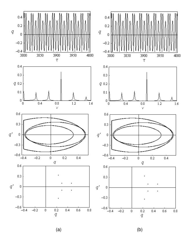
Figure 4.6. Time History Records, FFT Phase portraits, and Poincaré Maps for v = 0.88, and a = 0.104. Initial conditions  $z_o = 0.01$ ,  $z_o' = 0.01$ . (a) Elastic impact e = 1, and (b) Inelastic impact (Model 1) e = 0.8.
