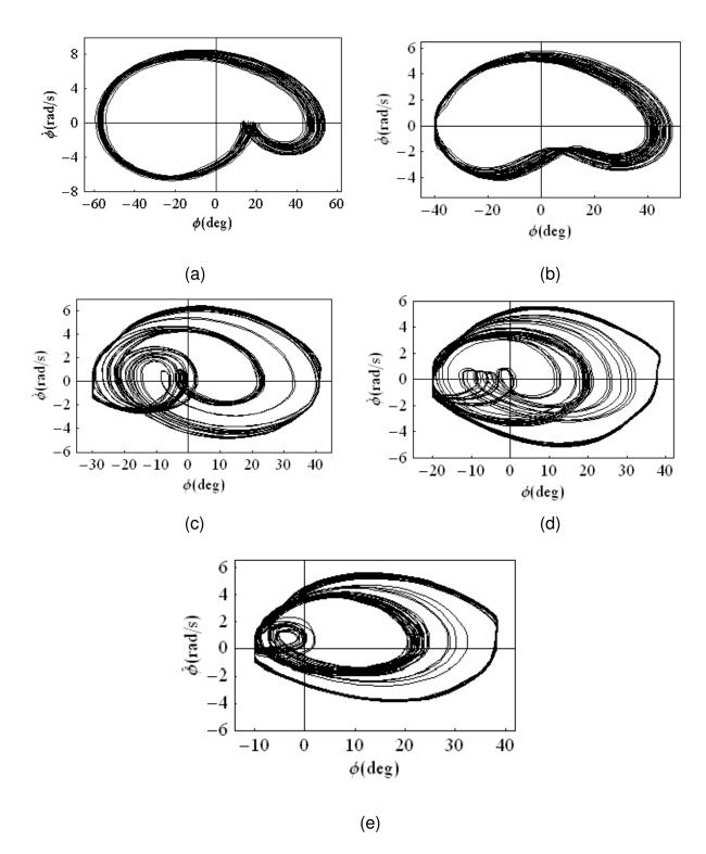
Figure 5.19. Phase trajectory projections of the model response shown in Figure 5.17 under motor speed  $N_m = 2.8 \text{ rad / s}$ : (a) in the absence of barrier, (b) in the presence of one-sided barrier at  $-40^\circ$ , (c) at  $-30^\circ$ , (d) at  $-20^\circ$ , (e) at  $-10^\circ$ .
