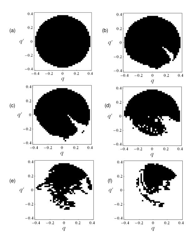
Figure 4.22. Domains of attraction for different excitation amplitudes for v = 0.88 as predicted by Model 2 for inelastic impact (e = 0.8); (a) a = 0.08, (b) a = 0.128, (c) a = 0.14, (d) a = 0.16, (e) a = 0.18, and (f) a = 0.22; Black region: bounded (safe) motion, and empty space: rollover dynamics.
