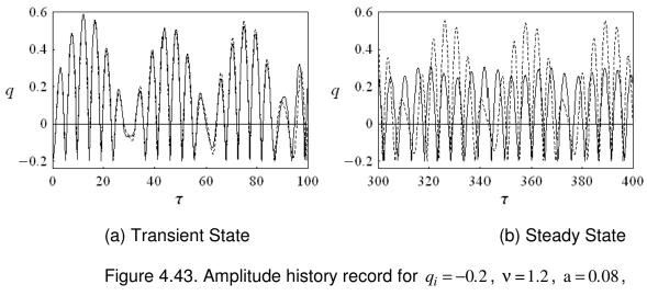
$z_o = 0.01, z_o' = 0.01$ , and e = 0.995; \_\_\_\_\_: Model 2, and \_\_\_\_: Equivalent damping method.
