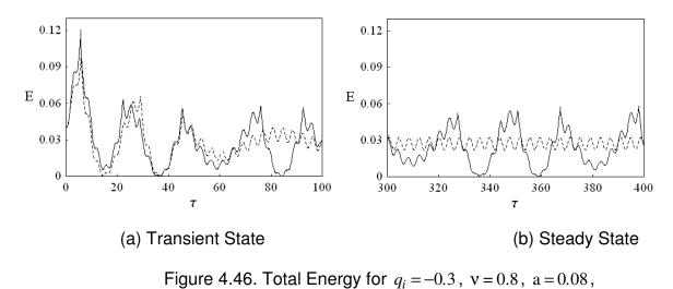
$z_o = 0.01, z_o' = 0.01$ , and e = 0.90; \_\_\_\_\_: Model 2, and \_\_\_: Equivalent damping method.
