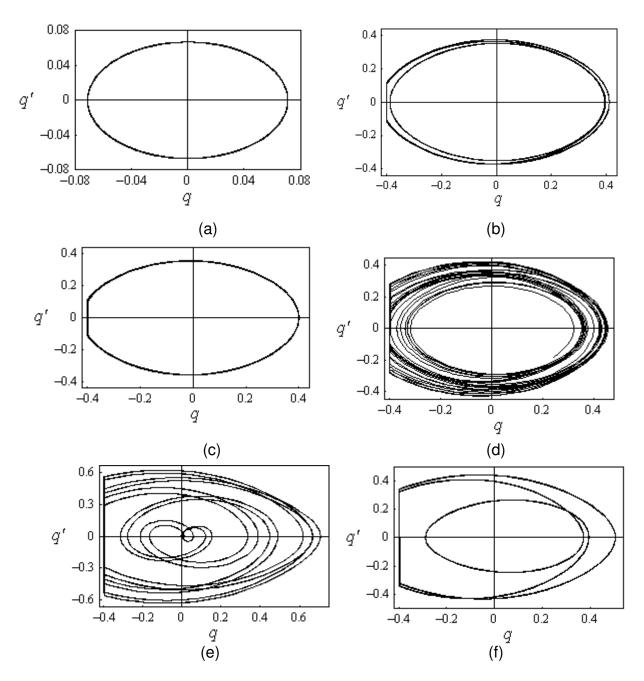
Figure 3.13. Phase portraits corresponding to the time history records of Figure 3.11 for excitation frequency ratio v = 0.94, and excitation amplitude: (a) a = 0.008, (b) a = 0.04 (period-two), (c) a = 0.06, (d) a = 0.07, (e) a = 0.096, and (f) a = 0.12 (period-three).
