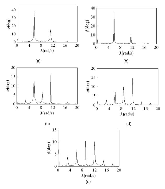
Figure 5.18. FFT plots of the model response shown in Figure 5.17 under motor speed  $N_m = 2.8 \text{ rad / s}$ : (a) in the absence of barrier, (b) in the presence of one-sided barrier at  $-40^\circ$ , (c) at  $-30^\circ$ , (d) at  $-20^\circ$ , (e) at  $-10^\circ$ .
