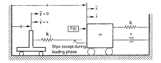
Figure 1.2. Skematic sketch of theoretical model by Sodhi (1991).
