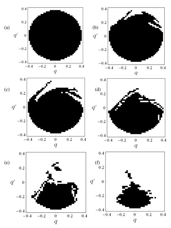
Figure 3.21. Domains of attraction for different excitation amplitudes for excitation frequency v = 1.2; (a) a = 0.04, (b) a = 0.056, (c) a = 0.064, (d) a = 0.08, (e) a = 0.104, and (f) a = 0.12; Black region: bounded (safe) motion, and empty space: rollover (unsafe)motion.
