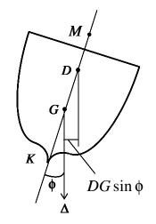
Figure 5.3. Determination of the vertical position of center of gravity of the ship model.
