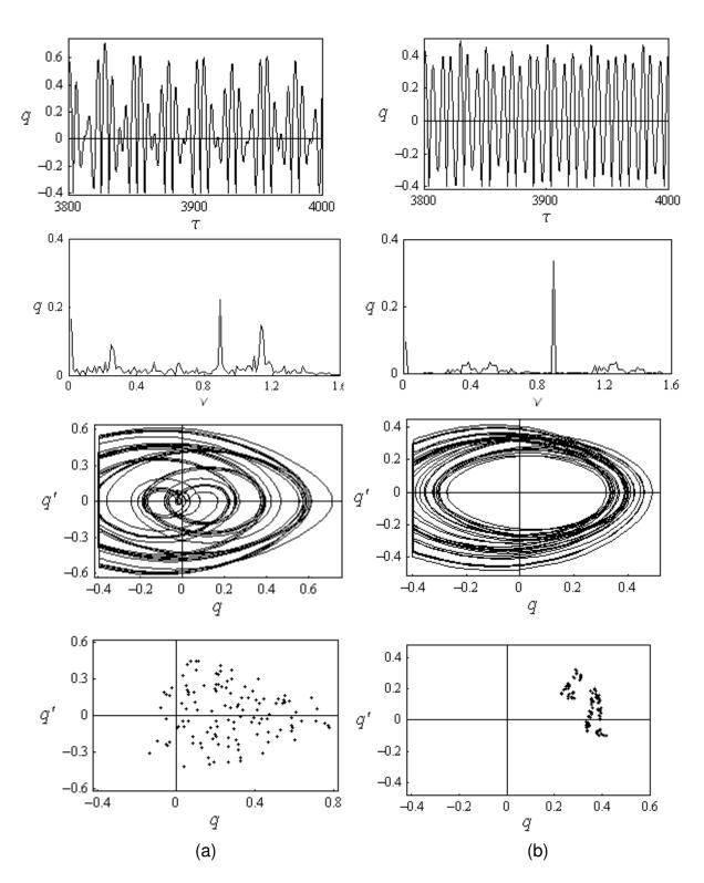
Figure 4.19. Ship time history records, FFT plots, phase portraits, and Poincaré Maps according to (a) Model 1, and (b) Model 2 for v = 0.88, a = 0.12, e = 0.8, and initial conditions  $z_o = 0.01$ ,  $z_o' = 0.03$ .
