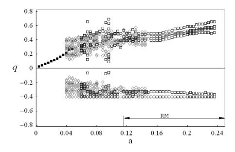
Figure 4.23. Bifurcation diagram for v = 0.88 as predicted by Model 2 for inelastic impact (e = 0.8); Period-one response,  $\Diamond$  Modulated response,  $\Box$  Multi - periodic response, and RM= Rollover Motion.
