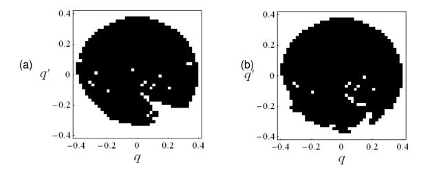
Figure 4.10. Domains of attraction for v = 0.88, and a = 0.104; (a) Elastic impact e = 1, and (b) Inelastic impact (Model 1) e = 0.8: Black region: bounded (safe) motion, and empty space: rollover dynamics.
