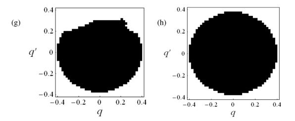
Figure 3.24. Domains of attraction for different excitation frequencies for excitation amplitude a = 0.08: (a) v = 0.6, (b) v = 0.92, (c) v = 0.96, (d) v = 1.0, (e) v = 1.12, (f) v = 1.2, (g) v = 1.28, and (h) v = 1.4; Black region: bounded motion, and empty space: rollover motion.
