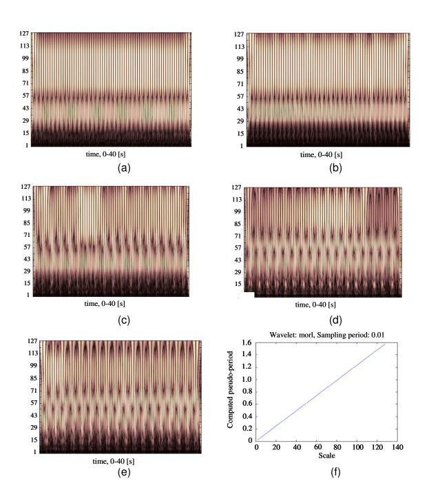
Figure 5.20. Morlet wavelet plots of the model response shown in Figure 5.16 under motor speed  $N_m = 2.8 \text{ rad/s}$ : (a) in the absence of barrier, (b) in the presence of one-sided barrier at  $-40^\circ$ , (c) at  $-30^\circ$ , (d) at  $-20^\circ$ , (e) at  $-10^\circ$ , and (f) shows the quasi period versus scale relationship.
