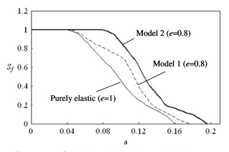
Figure 4.30. Safety factor diagram for excitation frequency v = 1.2; \_\_\_\_\_Purely elastic impact (*e*=1), and inelastic impact(*e*=0.8); \_\_\_\_\_Model 1, and \_\_\_\_\_Model 2.
