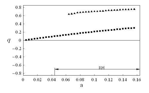
Figure 3.22. Bifurcation diagram for excitation frequency v = 1.2.
