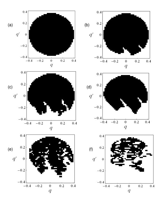
Figure 4.13. Domains of attraction for different excitation amplitudes for v = 0.94 as predicted by Model 1 for inelastic impact (e = 0.8); (a) a = 0.04, (b) a = 0.072, (c) a = 0.08, (d) a = 0.088, (e) a = 0.096, and (f) a = 0.104; Black region: bounded (safe) motion, and empty space: rollover dynamics.
