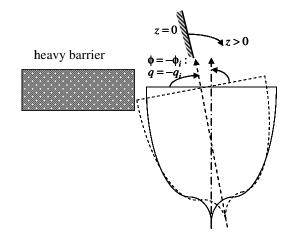
Figure 3.1. Schematic diagram of one-sided barrier impact with ship in roll oscillation.
