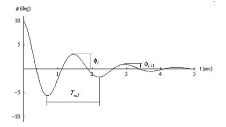
Figure 5.28. Free vibration test result.
