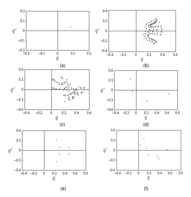
Figure 3.8. Poincaré maps corresponding to the time history records of Figure 3.5 for excitation frequency ratio v = 0.88, and excitation amplitude: (a) a = 0.02, (b) a = 0.046, (c) a = 0.084 (Chaotic), (d) a = 0.094 (Period four), (e) a = 0.106 (Period three), (f) a = 0.11 (Period seven).
