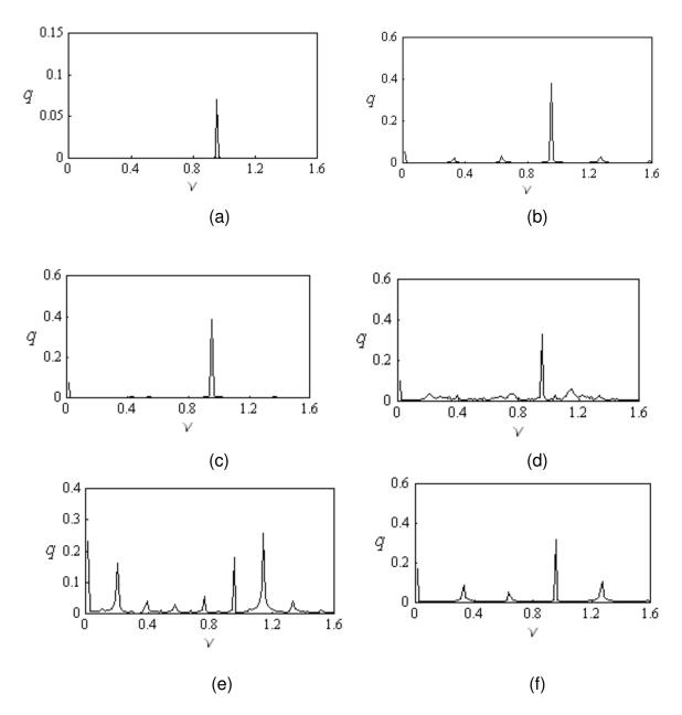
Figure 3.12. FFT corresponding to the time history records of Figure 3.11 for excitation frequency ratio v = 0.94, and excitation amplitude: (a) a = 0.008, (b) a = 0.04 (period-two), (c) a = 0.06, (d) a = 0.07, (e) a = 0.096, and (f) a = 0.12 (period-three).
