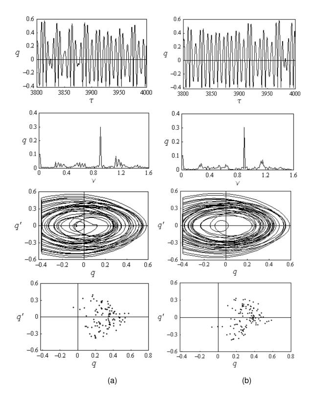
Figure 4.7. Time History Records, FFT, Phase portraits, and Poincaré Maps for v = 0.88, and a = 0.104. Initial conditions  $z_o = 0.15$ ,  $z_o' = -0.11$ . (a) Elastic impact e = 1, and (b) Inelastic impact (Model 1) e = 0.8.
