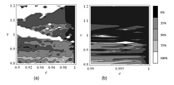
Figure 4.54. Contour Plot for error involved in equivalent damping method for a = 0.06,  $z_o = 0.01$ ,  $z_o' = 0.01$ , and  $q_i = -0.4$ : (a) e = 0.9 - 1.0, (b) e = 0.99 - 1.0.
