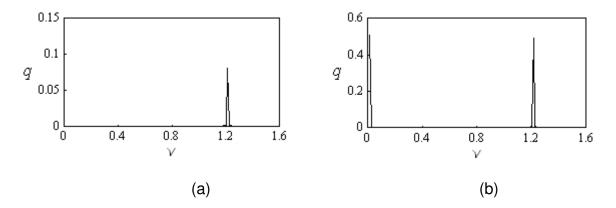
Figure 3.18. FFT corresponding to the time history records of Figure 3.17 for excitation frequency ratio v = 1.2, and excitation amplitude: (a) a = 0.036, and (b) a = 0.088.
