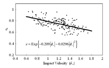
Figure 5.29. Dependence of the coefficient of restitution on the impact velocity (with the fitting curve is:  $e = \exp\left\{-0.209\left|\dot{\phi}_{-}\right| - 0.0296\left|\dot{\phi}_{-}\right|^{2}\right\}$
