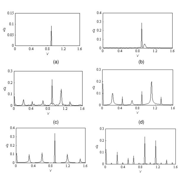
Figure 3.6. FFT corresponding to the time history records of Figure 3.5 for excitation frequency ratio v = 0.88, and excitation amplitude: (a) a = 0.02, (b) a = 0.046, (c) a = 0.084 (Chaotic), (d) a = 0.094 (Period four), (e) a = 0.106 (Period three), (f) a = 0.11 (Period seven).
