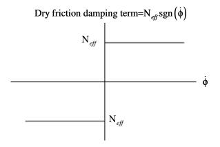
Figure 5.27. Dry friction damping term.
