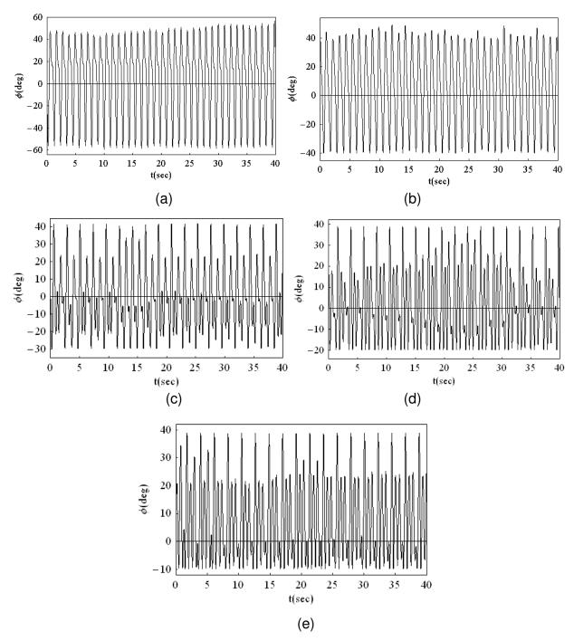
Figure 5.17. Measured time history records of the model response under motor speed  $N_m = 2.8 \text{ rad / s}$ : (a) in the absence of barrier, (b) in the presence of one-sided barrier at  $-40^\circ$ , (c) at  $-30^\circ$ , (d) at  $-20^\circ$ , (e) at  $-10^\circ$ .
