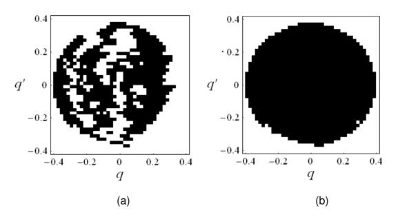
Figure 4.21. Domains of attraction according to (a) Model 1, and (b) Model 2 for v = 0.88, a = 0.12, e = 0.8, Black region: bounded (safe) motion, and empty space: rollover dynamics.
