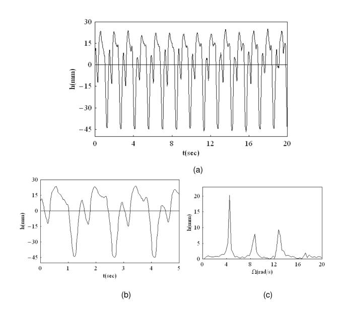
Figure 5.21. Free surface wave at wave maker motor speed  $N_m = 2.2$  rad/s : (a) time history record of the water free surface, (b) magnification of few cycles showing the wave profile, and (c) FFT plot.
