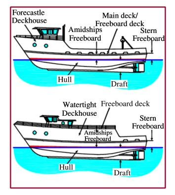
Figure A.1. Key parts of a ship structure.
