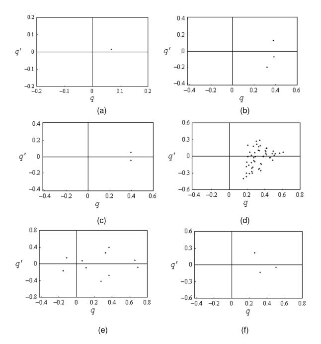
Figure 3.14. Poincaré maps corresponding to the time history records of Figure 3.11 for excitation frequency ratio v = 0.94, and excitation amplitude: (a) a = 0.008, (b) a = 0.04 (period-two), (c) a = 0.06, (d) a = 0.07, (e) a = 0.096, and (f) a = 0.12 (period-three).
