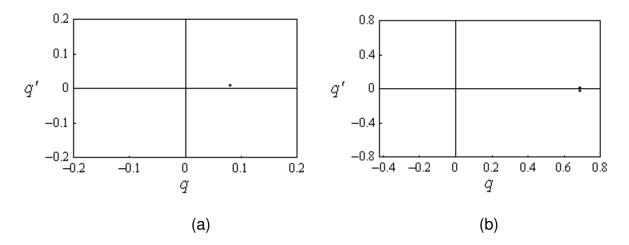
Figure 3.20. Poincaré maps corresponding to the time history records of Figure 3.17 for excitation frequency ratio v = 1.2, and excitation amplitude: (a) a = 0.036, and (b) a = 0.088.
