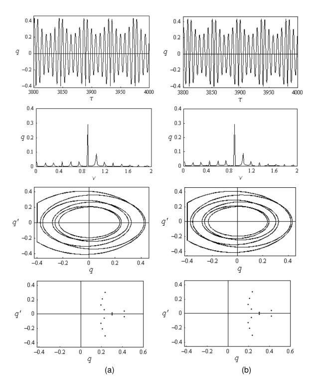
Figure 4.2. Time History Records, FFT, Phase portraits, and Poincaré Maps for v = 0.88, and a = 0.06. Initial conditions  $z_o = 0.01$ ,  $z_o' = 0.01$ . (a) Elastic impact e = 1, and (b) Inelastic impact (Model 1) e = 0.8.
