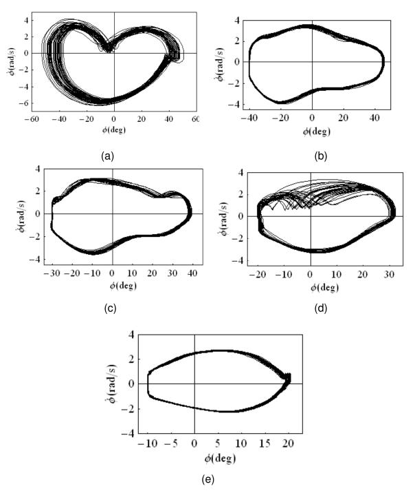
Figure 5.15. Phase trajectory projections of the model response of Figure 5.13 under motor speed  $N_m = 2.4$  rad/s : (a) in the absence of barrier, (b) in the presence of one-sided barrier at  $-40^\circ$ , (c) at  $-30^\circ$ , (d) at  $-20^\circ$ , (e) at  $-10^\circ$ .
