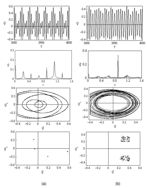
Figure 4.17. Ship time history records, FFT plots, phase portraits, and Poincaré Maps according to (a) Model 1, and (b) Model 2 for v = 0.88, a = 0.084, e = 0.8, and initial conditions  $z_0 = 0.01$ ,  $z'_0 = 0.01$ .
