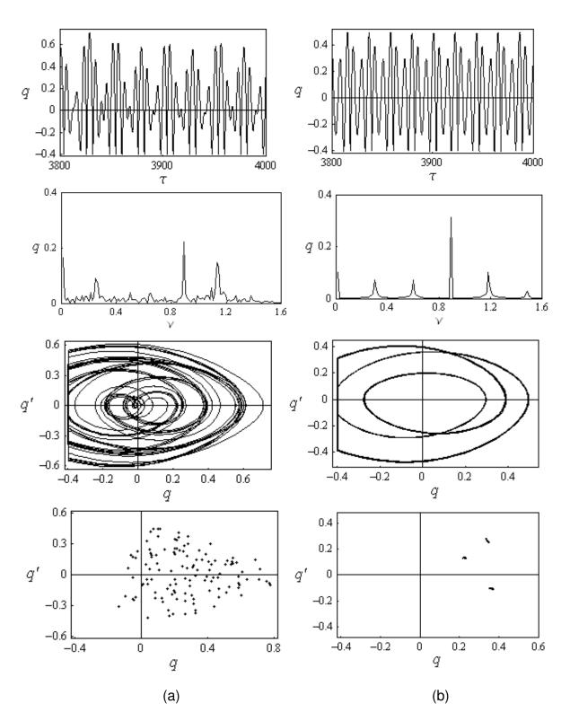
Figure 4.18. Ship time history records, FFT plots, phase portraits, and Poincaré Maps according to (a) Model 1, and (b) Model 2 for v = 0.88, a = 0.12, e = 0.8, and initial conditions  $z_o = 0.01$ ,  $z_o' = 0.01$ .
