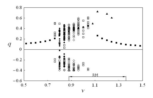
Figure 3.25. Amplitude versus excitation frequency diagram for excitation amplitude a = 0.08: ■ Period-one response, ▲ Period-one response experiencing impact, △ Period-two Response, ◇ Modulated response, □ Multi - periodic response, ● Chaotic motion, and RM= Rollover Motion.
