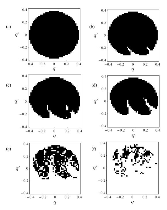
Figure 3.15. Domains of attraction for different excitation amplitudes for excitation frequency v = 0.94; (a) a = 0.04, (b) a = 0.072, (c) a = 0.08, (d) a = 0.088, (e) a = 0.096, and (f) a = 0.104; Black region: bounded (safe) motion, and empty space: rollover dynamics.
