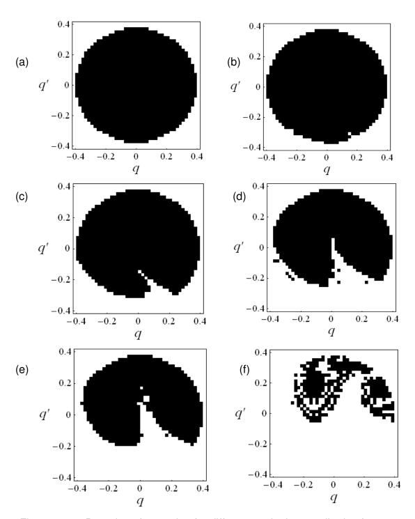
Figure 4.25. Domains of attraction for different excitation amplitudes for v = 0.94 as predicted by Model 2 for inelastic impact (e = 0.8); (a) a = 0.088, (b) a = 0.096, (c) a = 0.104, (d) a = 0.12, (e) a = 0.128, and (f) a = 0.136; Black region: bounded (safe) motion, and empty space: rollover dynamics.
