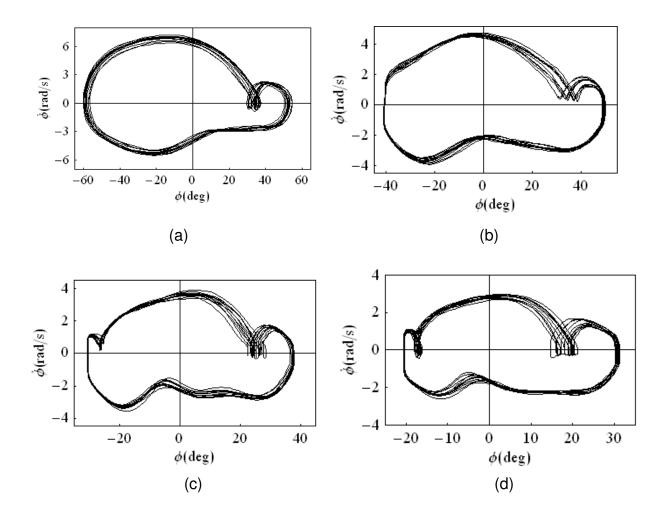
Figure 5.24. Phase trajectory projections of the model response of Figure 5.22 under motor speed  $N_m = 2.2 \text{ rad/s}$ : (a) in the absence of barrier, (b) in the presence of one-sided barrier at  $-40^\circ$ , (c) at  $-30^\circ$ , and (d) at  $-20^\circ$ .
