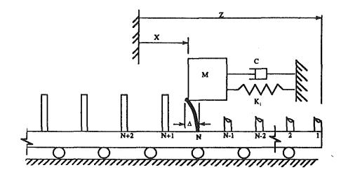
Figure 1.1. Skematic sketch of the theoretical model by Matlock (1971).
