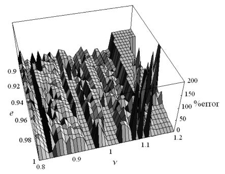
Figure 4.49. Error involved in equivalent damping method as a function of excitation frequency ratio v and coefficient of restitution e for a = 0.08,
