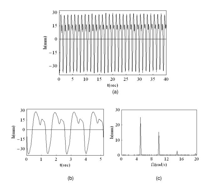
Figure 5.12. Free surface wave at wave maker motor speed  $N_m = 2.4$  rad/s : (a) time history record of the water free surface, (b) magnification of few cycles showing the wave profile, and (c) FFT plot.
