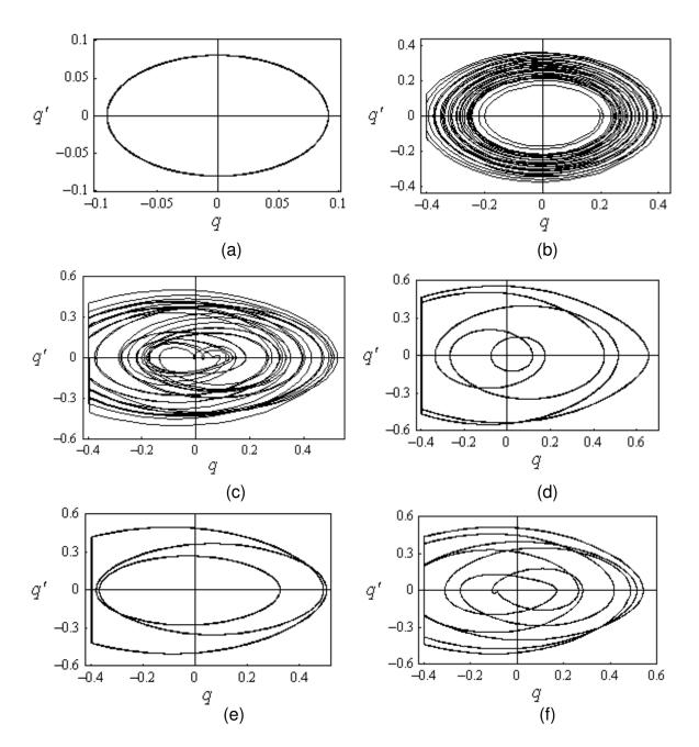
Figure 3.7. Phase portraits corresponding to the time history records of Figure 3.5 for excitation frequency ratio v = 0.88, and excitation amplitude: (a) a = 0.02, (b) a = 0.046, (c) a = 0.084 (Chaotic), (d) a = 0.094 (Period four), (e) a = 0.106 (Period three), (f) a = 0.11 (Period seven).
