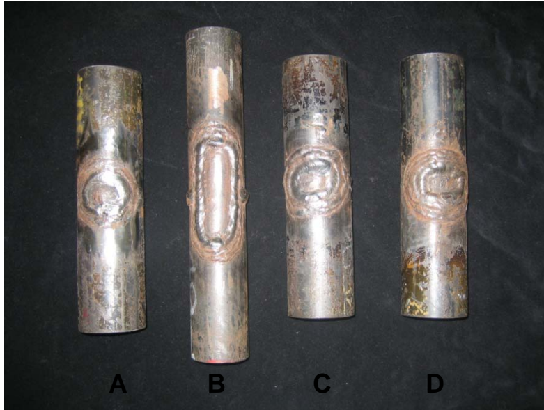
Figure 3.17: Sample boiler tubes used in experiment
