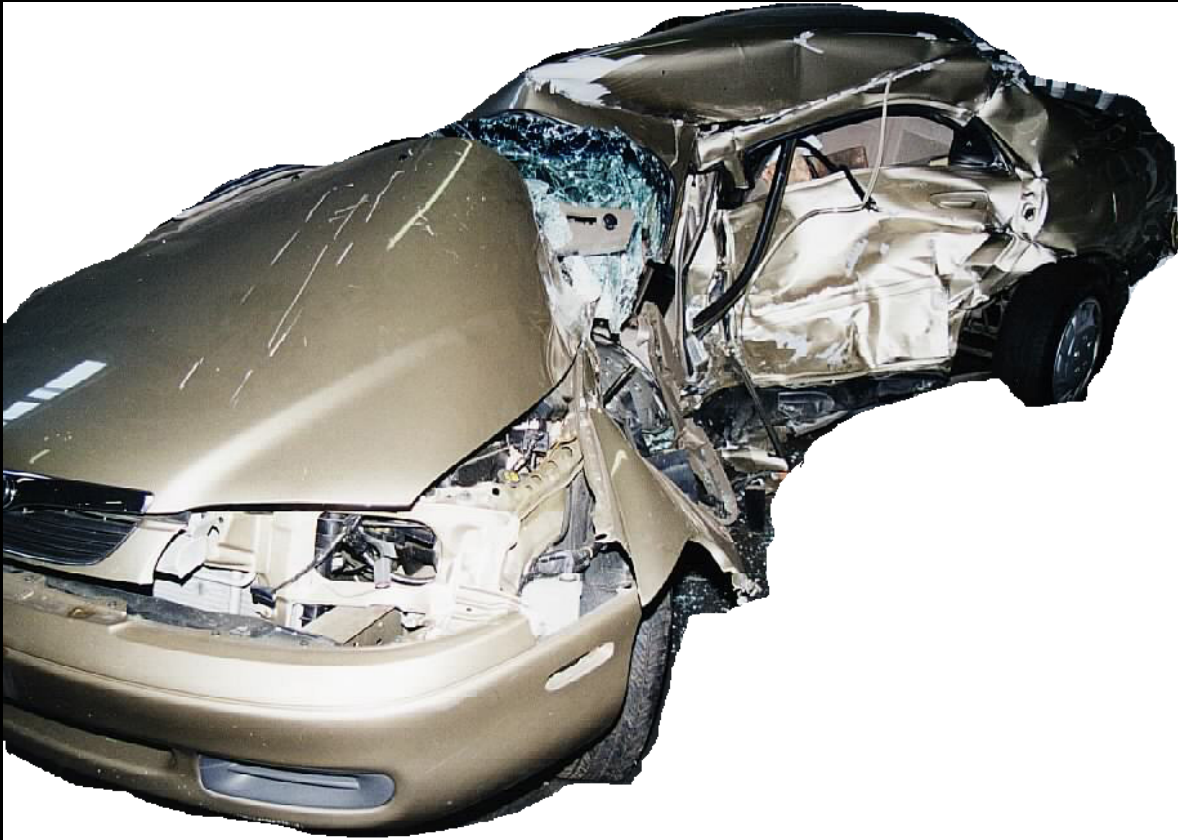
Figure 4.20: Deformation pattern of the struck vehicle, case#16
