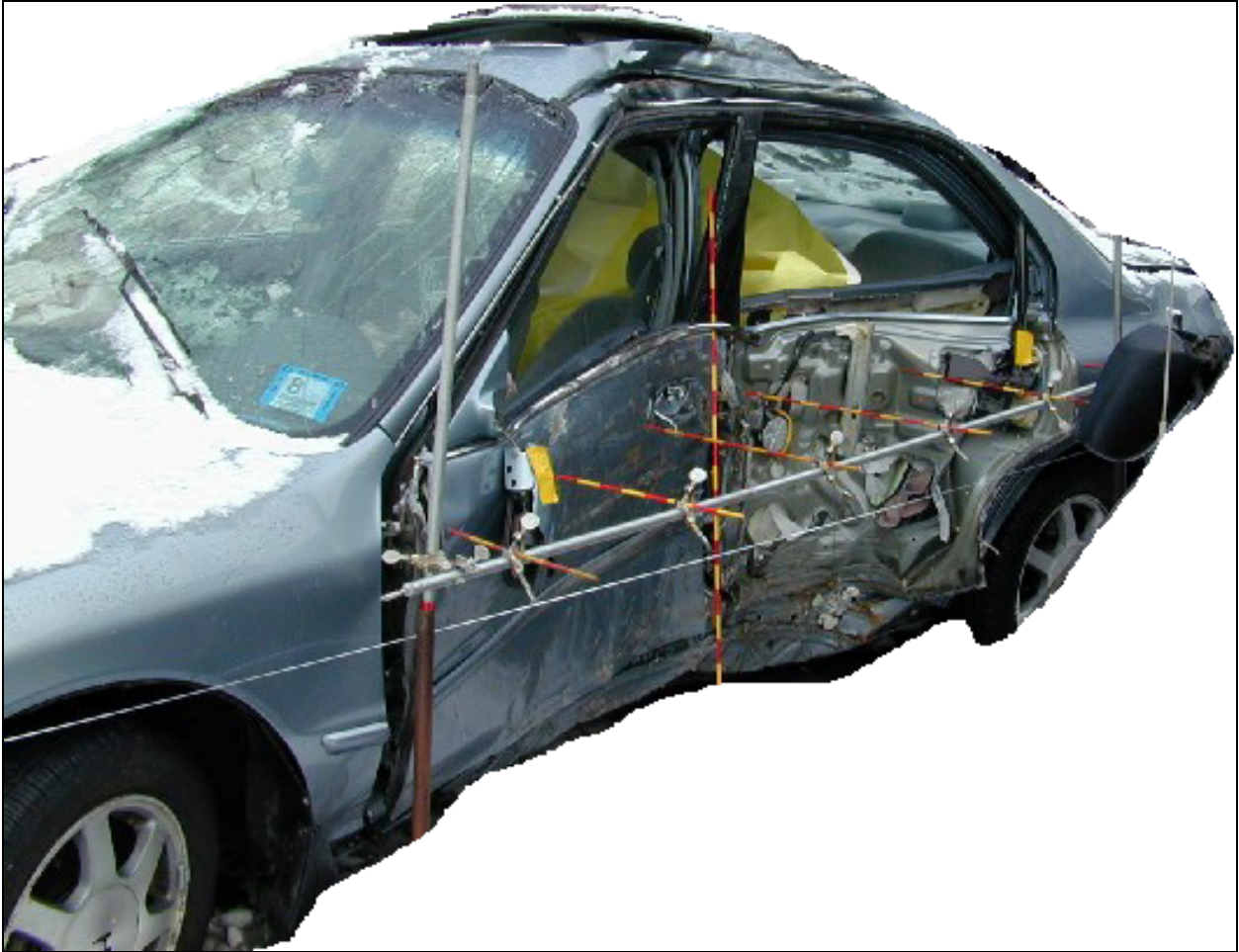
Figure 4.14: Deformation pattern of the struck vehicle, case#8
