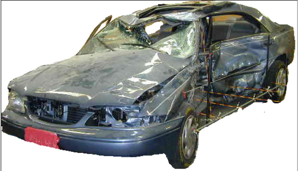
Figure 4.8: Deformation pattern of the struck vehicle, case#6
