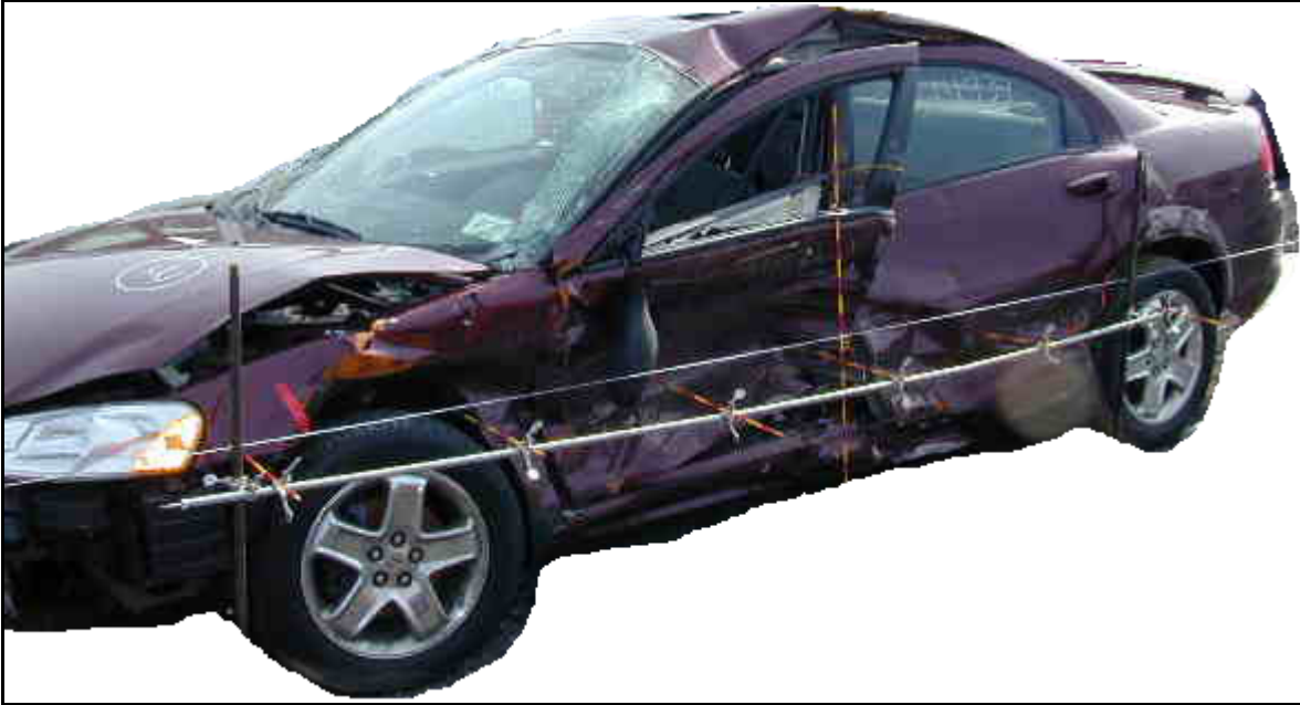
Figure 4.23: Deformation pattern of the struck vehicle, case#17
