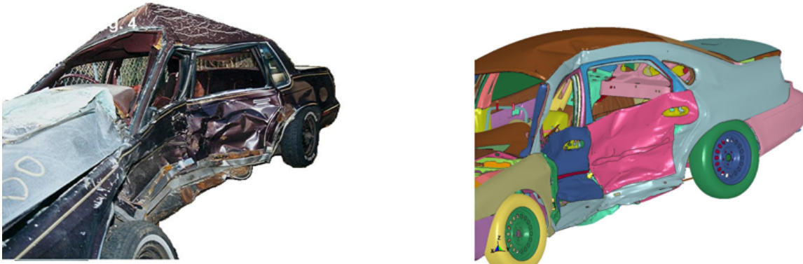
Figure B6: Vehicle deformation comparison of simulated FE vehicle against actual vehicle – CASE 15
