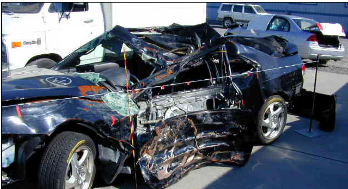
Figure 4.5: Deformation pattern of the case vehicle, case #5
