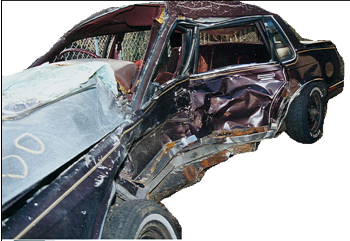
Figure 4.17: Deformation pattern of the struck vehicle, case#15
