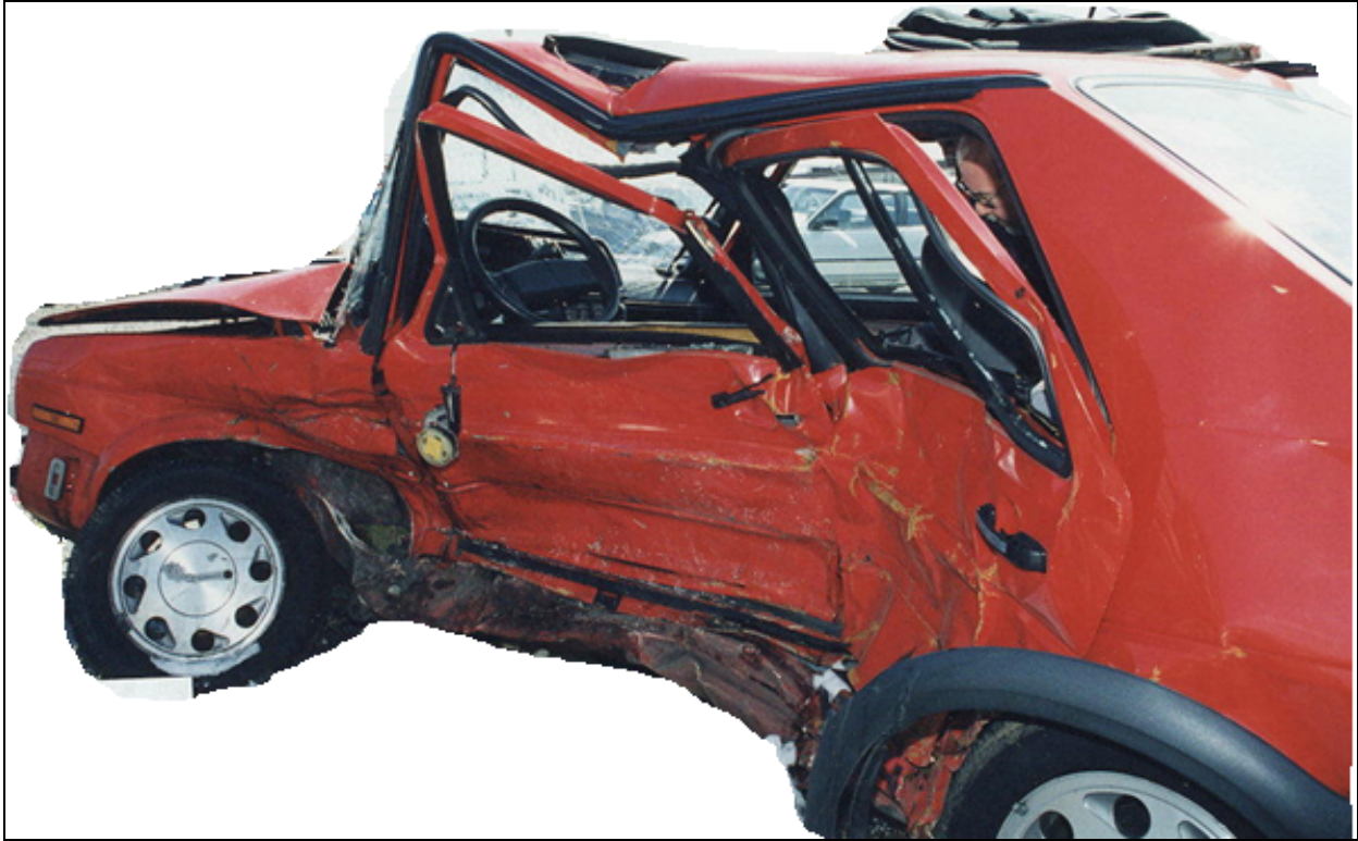
Figure 4.2: Deformation pattern of the struck vehicle, case #4
