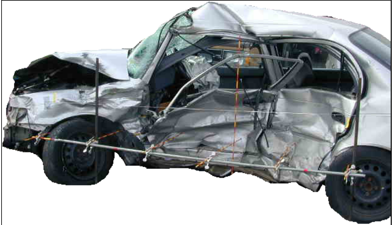
Figure 4.11: Deformation pattern of the struck vehicle, case#7
