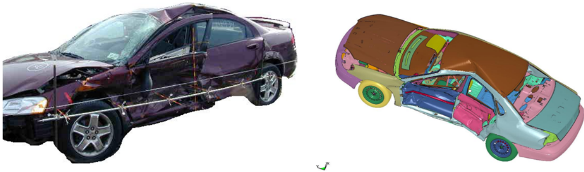
Figure B8: Vehicle deformation comparison of simulated FE vehicle against actual vehicle – CASE 17
