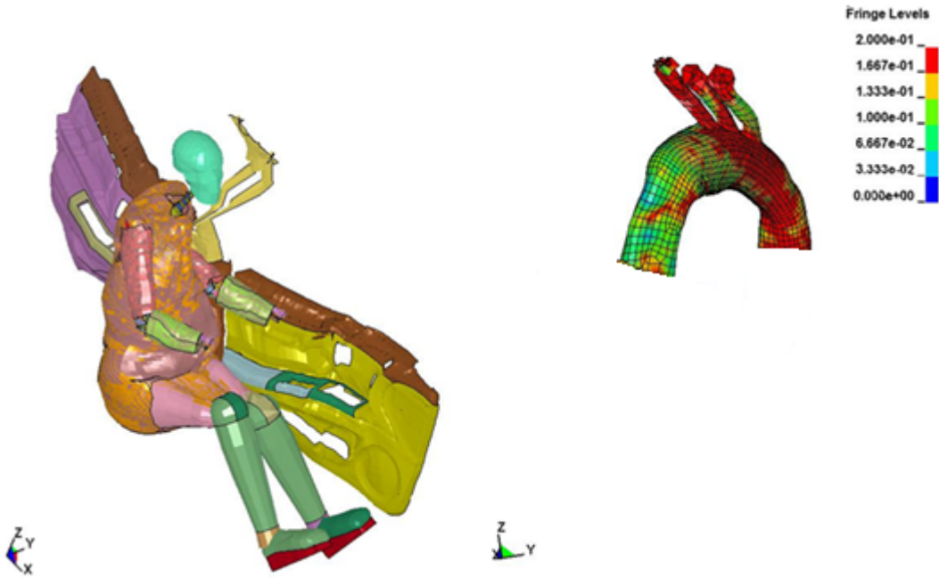
Figure B11: (a) Occupant kinematics and (b) Maximum principal strain pattern at the time of maximum vehicle deformation – CASE 6
