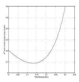
Figure 41: Closed-loop system performance vs. filter decaying rates
