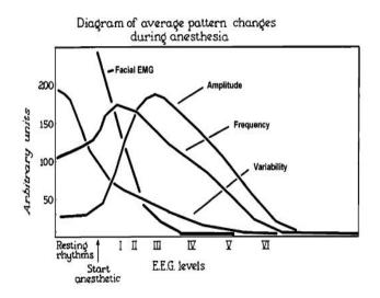
Figure 2: Changes of several EEG and EMG parameters as anesthesia is deepened nized with the thalamic pacemaker. Finally, the EMG of the frontal muscles disappears as the anesthesia deepens. Based on these observations the EEG may be capable of reflecting a gradual change in anesthetic effect by using a combination of EEG amplitude, frequency, variability, topography, and frontal EMG.
