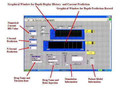
Figure 29: Front panel of the simple version system
