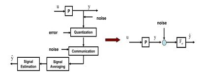
Figure 35: Signal filtering in open-loop systems
