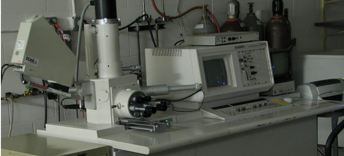
Figure 1-2 Hitachi S-2400 SEM in Laboratory of Analytical Electron Microscopy (LAEM)
