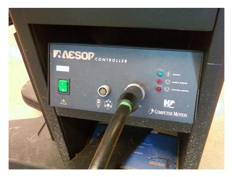
Figure 5-2: AESOP 1000 motion controller
