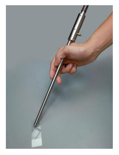
Figure 3-3: Raman spectroscopy probe
