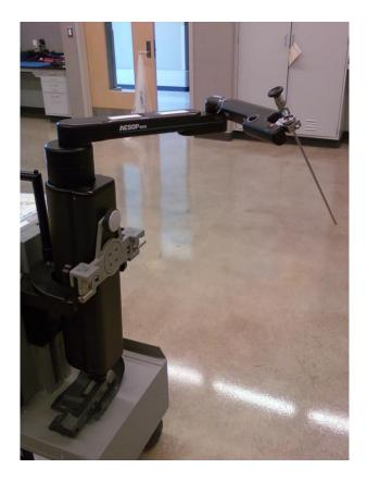
Figure 5-1: AESOP 1000 robotic arm
