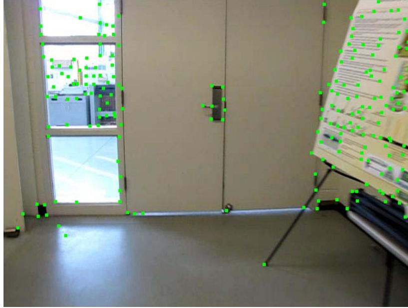
Figure 8: The "good features" to track that were found running OpenCV's implementation of Shi and Tomasi's algorithm.
