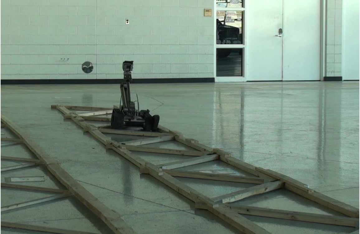
Figure 50: The PackBot going over the 2x4 course during subject testing.
