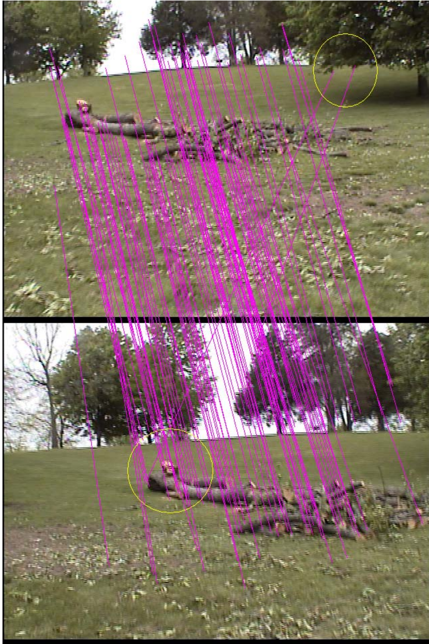
Figure 21: An example of matching SIFT features from two Images from the “wood pile” dataset. The yellow ellipses show where the SIFT algorithms made obvious mismatches.
