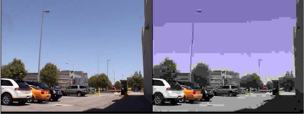
Figure 3: The image on the left is an image obtained directly from an analog camera. The image on the right is the same image with 90% JPEG compression applied.
