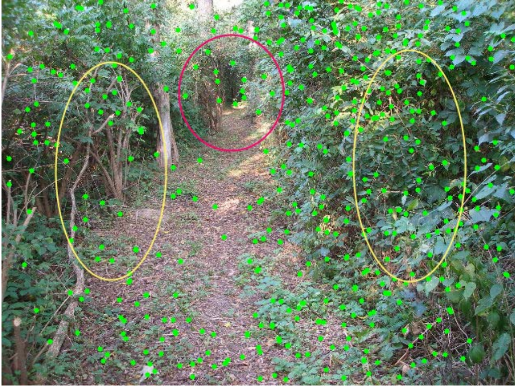
Figure 12: An image of wooded path. The green points were found using Shi and Tomasi's corner detector. The points contained in the yellow ellipses have greater motion as the robot moves forward than the points in the red ellipse.
