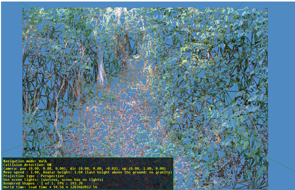
Figure 13: This is the same wooded scene shown earlier but with the 3D facets found using Make3D shown.
