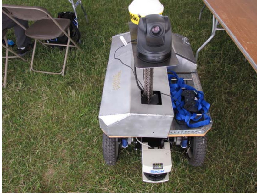
Figure 24: The IGVC platform that was equipped with a camera, GPS, and an IMU for data collection.
