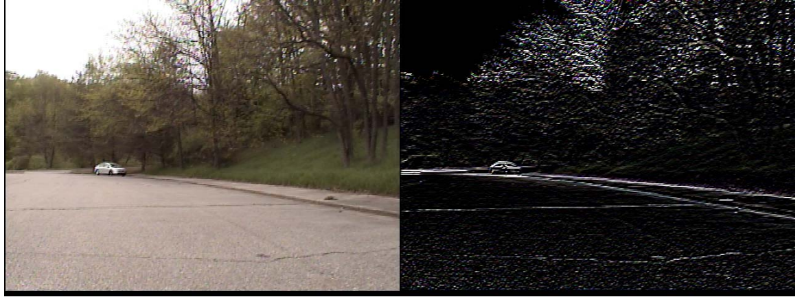
Figure 7: The results of the Sobel operator running on an image.
