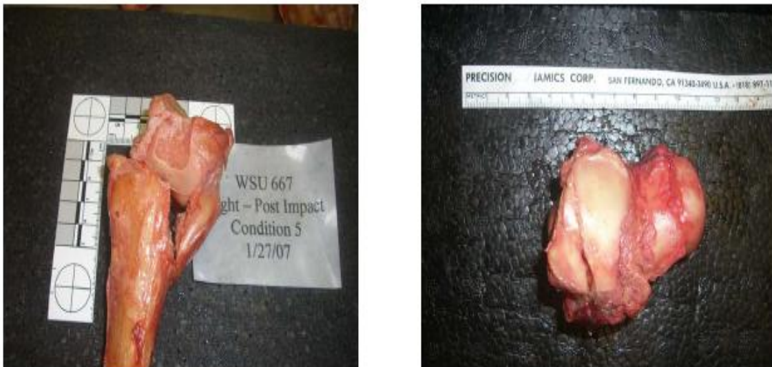
Figure 30: Left: Medial Malleolus Fracture. Right: Posterior Calcaneal Articular Surface Fracture.
