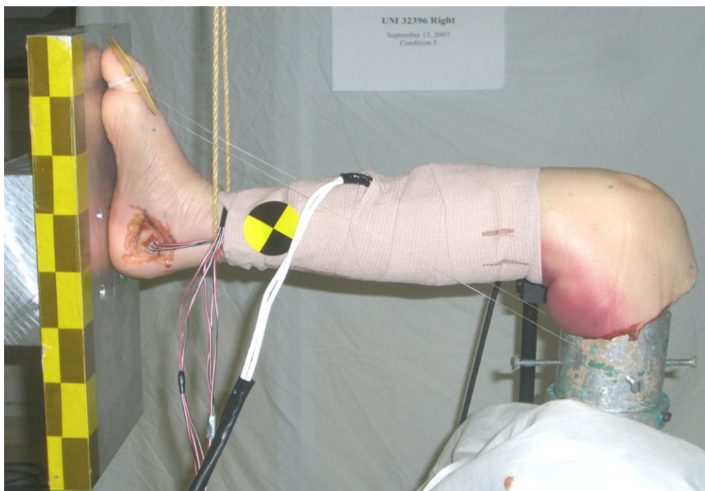
Figure 27: Positioning of Instrumented PMHS Lower Extremity Prior to Impact.
