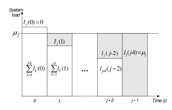
Figure 5.2: Illustration of the optimal time-variant resource allocation for queue *j*.
