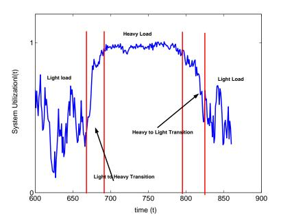
Figure 4.10: System utilization process under an input of video traffic.
