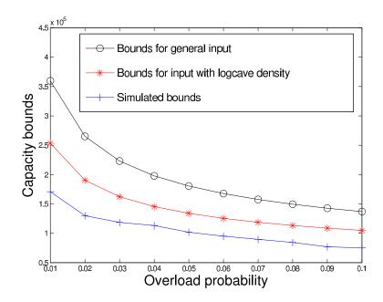
Figure 6.4: Capacity bounds for inputs with unimodal distribution.
