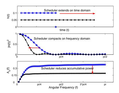
Figure 3.4: Trade-off between length of scheduler h(t), width of EDS function  $|H(f)|^2$  and value of CPF function  $A_h(f)$
