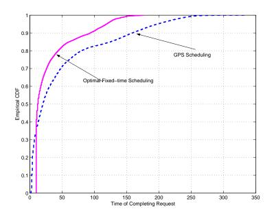
Figure 4.5: The CDF plot of completion time when  $n(t) \sim ln(1, 2)$
