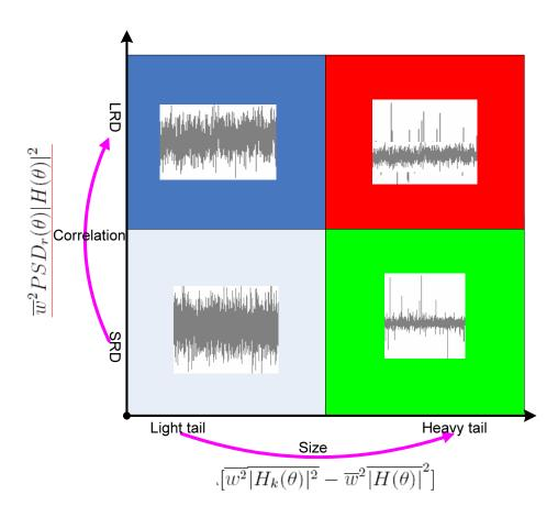
Figure 3.7: Map of four regions [78] in traffic dynamics to server workload dynamics with workload equation 3.42 for decay function modulated point process .
