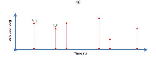
Figure 3.5: An illustration of marked random point process.
