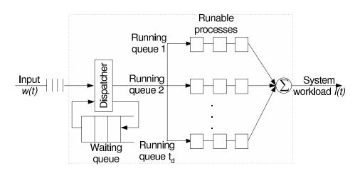
Figure 5.1: Decay function model with multiple queues to support service differentiation
