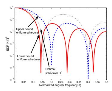
Figure 6.5: The illustration of upper bound and lower bound for server optimal scheduling function. Through convex scheduling and minimum power theorems, an optimal scheduler can be bounded by the uniform scheduler with same service deadline and a uniform scheduler with longer service deadline.
