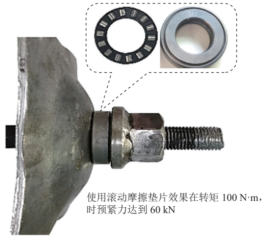
图 5 滚动式减摩垫片 TX1 Fig.5 Rolling anti-friction gasket TX1
