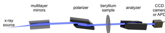
Figure 13: Sketch of the experimental setup investigating CRL material properties. The multilayer mirrors collimate the X-rays from the rotating anode X-ray source. The combination of the polarizer, analyzer, and CCD camera allows for polarization sensitive imaging. Taken from Grabiger et al. [61] .
