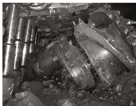
(a) Coal mining machine rocker arm breakage
