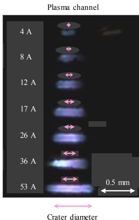
Fig. 6. Images of plasma channels at different currents [10].
