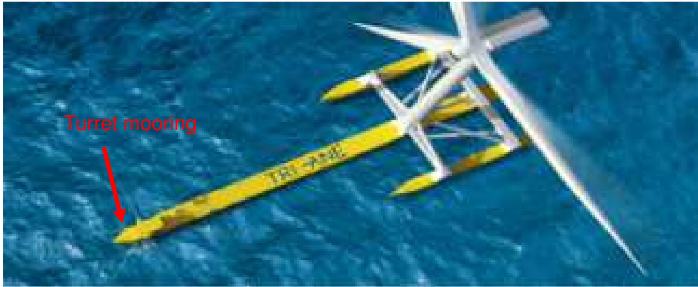
Model test University of Plymouth scale 1/50
