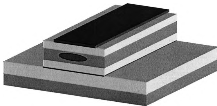
Fig. 4.3 Deeply-etched waveguide electrooptic GaAs modulator, Mach-Zehnder part.
