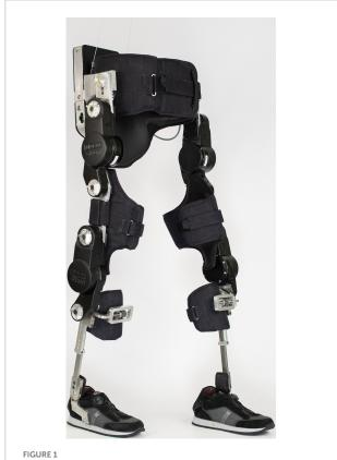
The TWIN lower limb exoskeleton.
