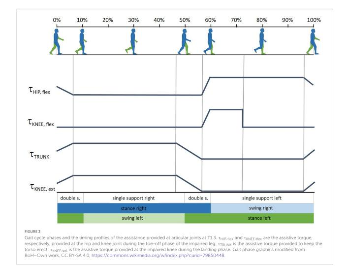
stance phase ( $\tau_{TRUNK}$  in **Figure 4**); (iii) stabilization of the knee joint of the support leg during both stance phases ( $\tau_{KNEE,ext}$  in **Figure 4**); and (iv) hip extension support of paretic leg during stance phase ( $\tau_{HIP,ext}$  in **Figure 4**).
