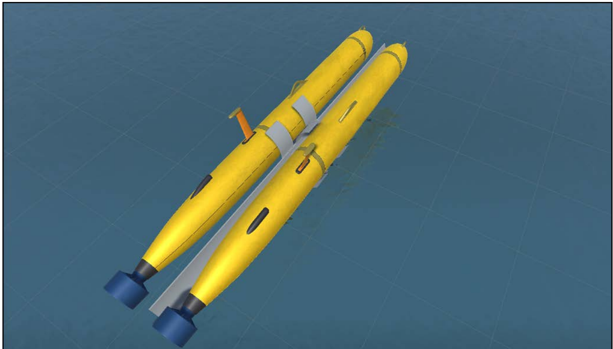
Figure 1: Automated Revolver able to Deploy 3 AUV (Autonomous Underwater Vehicle)
