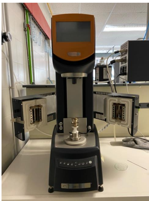
Figure 3.6. HR 10 rheometer from TA Instruments used for the rheological characterization of the materials.
