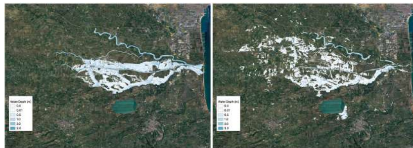
Figure 12. Water depths maps for the Catanian floodplain (Sicily) from TELEMAC-2D (left panel) and FwDET tool (right panel).
