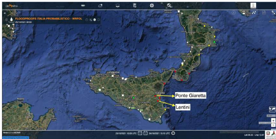
Figure 5. FloodPROOFS forecast over southern Italian rivers sections. Visualization on MyDewetra platform. The different sections' colors refer to the magnitude of the peak discharge with respect to the fixed threshold for alarm (yellow) and alert (red). Green and white colors refer to discharge increasing but still below thresholds and discharge not increasing or decreasing, respectively.
