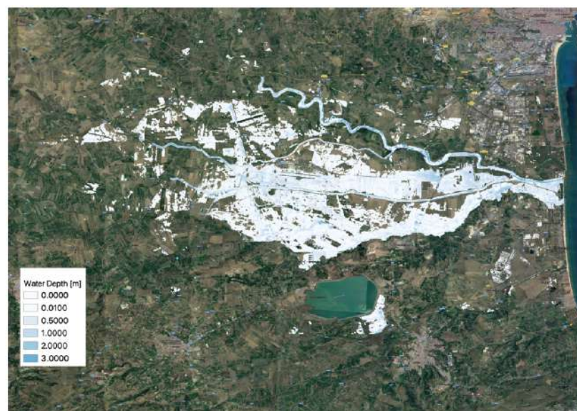
Figure 13. Water depth map obtained for the Catanian floodplain (Sicily) from the merging of TELEMAC-2D and FwDET tool results.
