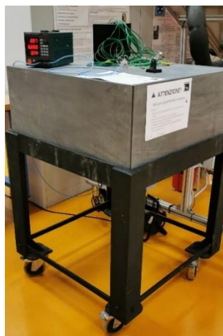
Figure 70. The rock sample (slate) and the cart that is used to keep the block stably raised during the planned experimental activity.
