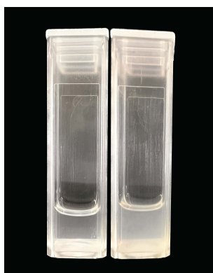
Figure 3.12 – Macroscopic evidence of the effect of surfactant on the stability of colloidal suspensions. On the left, there is a cuvette containing a solution containing just Gd 2 O 3 NPs in 2-butanone, while on the right there is a cuvette containing Gd 2 O 3 NPs treated with Igepal in 2-butanone. With the same concentration of NPs, the solution on the right appears more opaque, while the other is more clear, and this is symptomatic of the sedimentation of the NPs.
