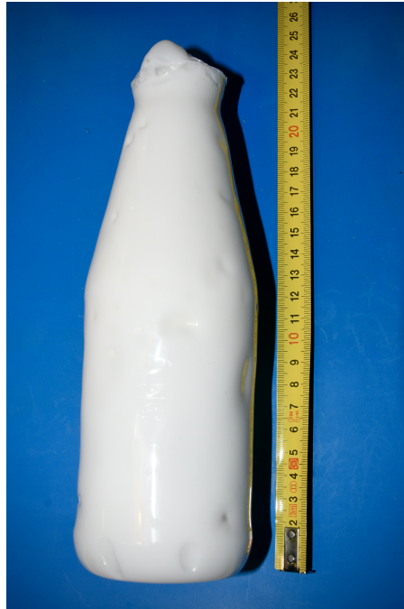
Figure 3.17 – One of the most satisfactory samples produced during the R&D: a 23 cm height sample with a uniform concentration of 1% w Gd 2 O 3 .
