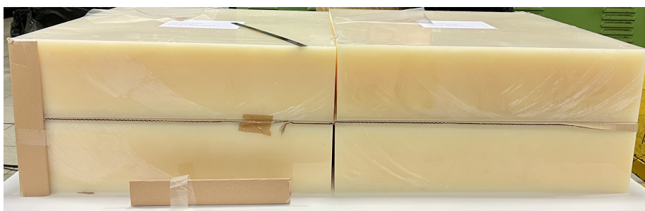
Figure 6.5 – Industrial samples Clax 1-1, Clax 1-2, Clax 1-3, and Clax 1-4. As can be seen, all have a yellowish color towards the center. On the side faces it is possible to notice the signs of the standard mechanical processes (not optimized for the experiment) that the company operates after production.
