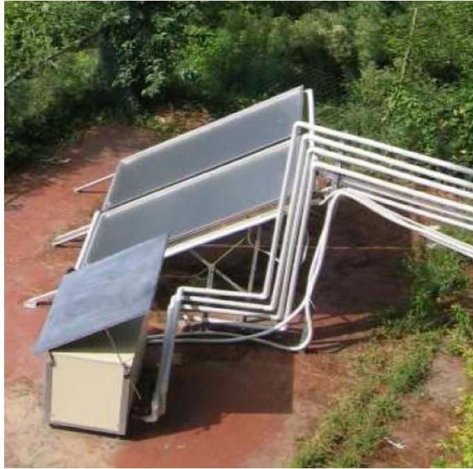
Figure 2. 3: prototype of solar assisted heat pump with hybrid panels at Cus Genova (21)
