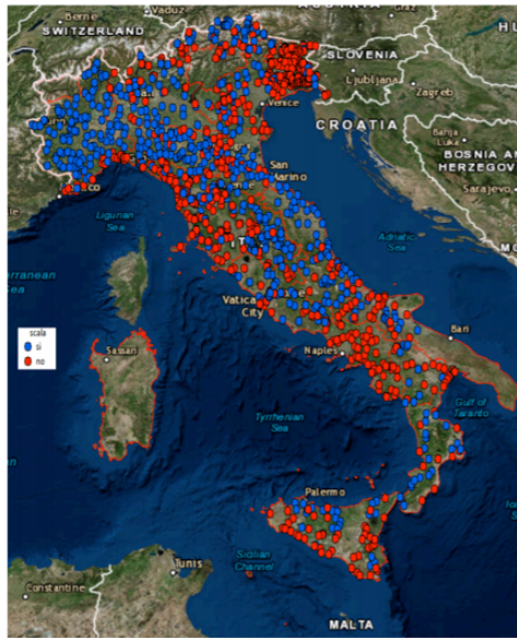
Figure 2.7: Water level gauges across Italy with (blue dots) and without (red dots) updated rating curves as of 2016, from [121].
