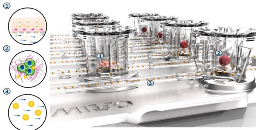
Figure 52: Dynamic multi-organ platform. A novel multi-organ-on-chip configuration was developed to co-culture HepG2 cells monolayers in one chamber (1) and ovarian cancer 3D hydrogel-based models
